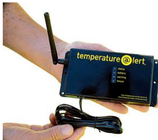
Figure 4. Cellular Temperature Monitoring System
