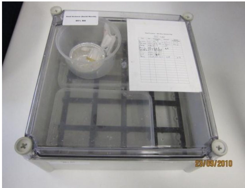
Figure 1. Sealed Polycarbonate Electrical Enclosure or Box Used to Store Seeds (Photo from Dr. J. Walck, Dept. of Biology, MTSU)
