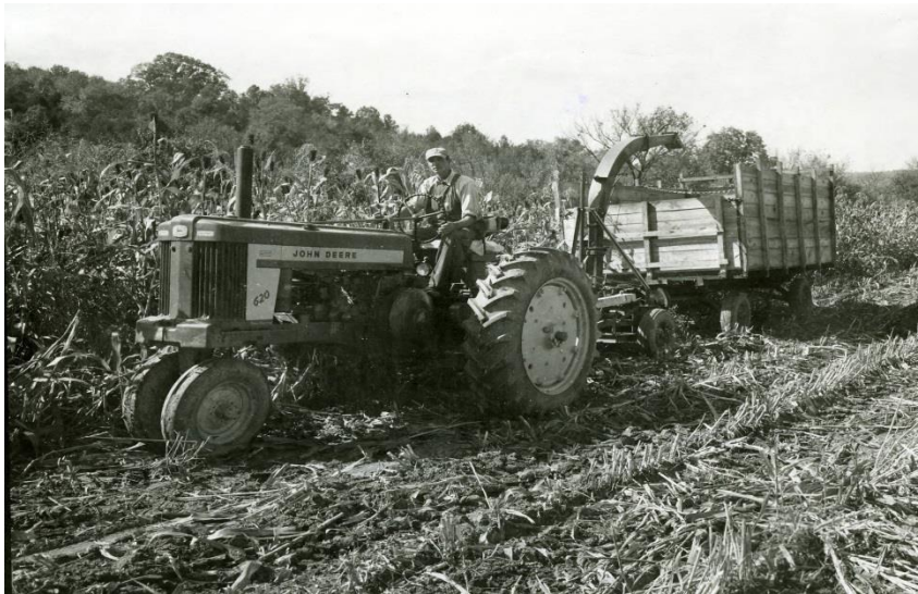
Figure 13. Harvesting corn and sorghum for silage , 10-06-1958. Photographer's note: "Paul Todd operating tractor and pulling silage chopper. Silage being made from a mixture of corn and sorghum then stored in trench silo with concrete sides and bottom. Chopper and wagons owned jointly by four farmers and two other newly constructed concrete trench silos have been tilled this year with the equipment. Excellent crop of silage on Huntington and Mimosa soil. Located two miles south of Woodbury. Source : Cannon County, Tennessee Farms, Walker Library at MTSU, Digital Collections.
