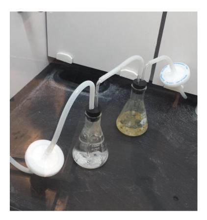
**Figure 4:** Experimental bubble bioreactor system overview. Oxygen flows from the left of the picture through a sterile filter into a hydration chamber filled with sterile deionized H<sub>2</sub>O. Oxygen is then directed through a growth chamber containing cells and media and is released after passing an additional sterile filter. System kept in a fume hood setting (sterilized with 70% isopropyl alcohol) at room temperature
