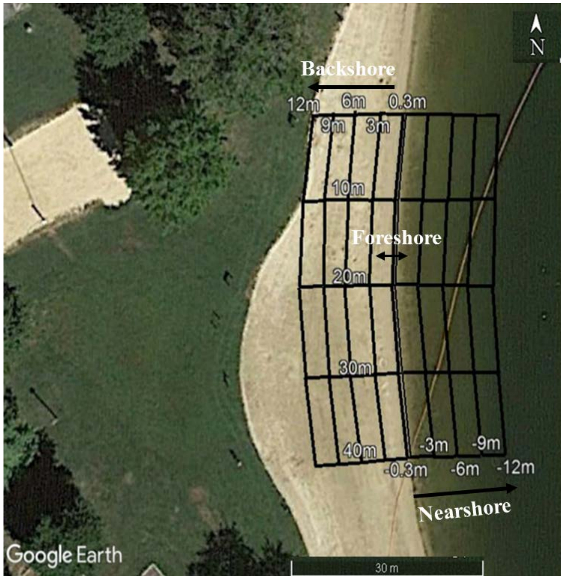
Figure 4.1. Sampling transect for sand core samples taken at Cedar Creek Recreational Area, Tennessee. Samples were taken at points where two lines intersect. Backshore (3, 6, 9, 12 m), foreshore (0.3 to -0.3 m), and nearshore (-3, -6, -9, -12 m) areas are indicated by arrows.
