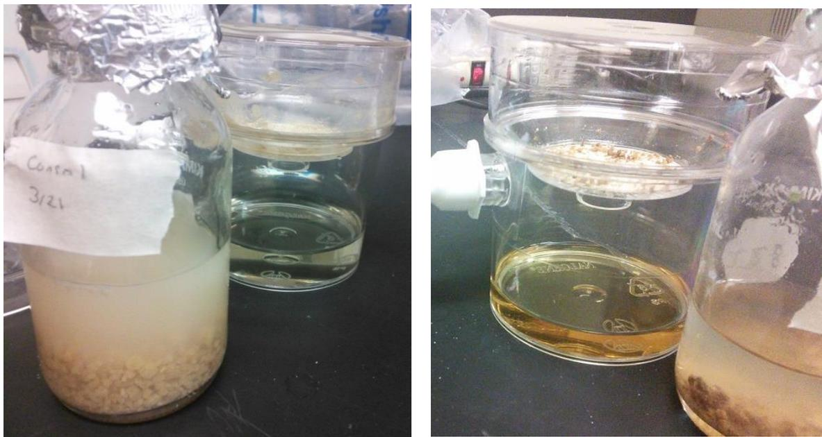
**Figure 13:** Filtered media from shaker suspension culture (left) and experimental bubble bioreactor (right). Bottles contain cell masses extracted from filtered suspensions
