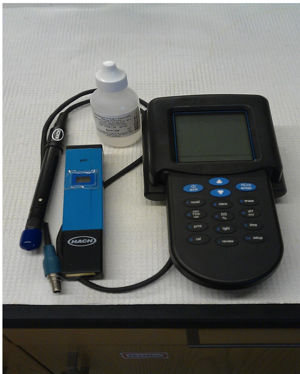
Figure 1. BOD 5 Analysis Setup: DO Meter, Probe And pH Meter
