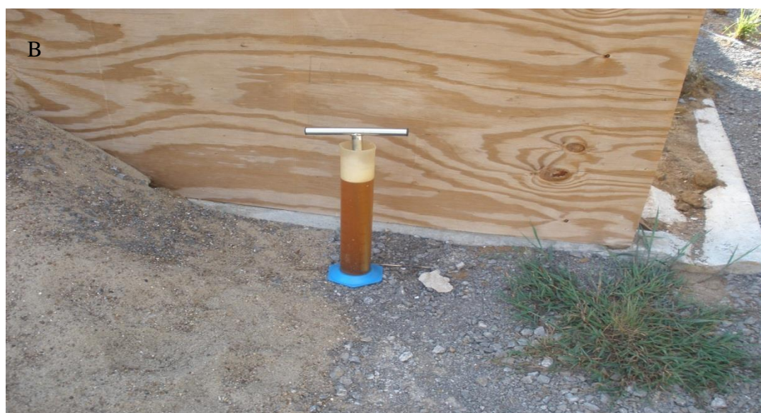
Figure 2. Core sampling. (A) One of three compost core samplers used in the first summer trial. (B) Core sampler decontamination with a 10% Lysol® solution.
