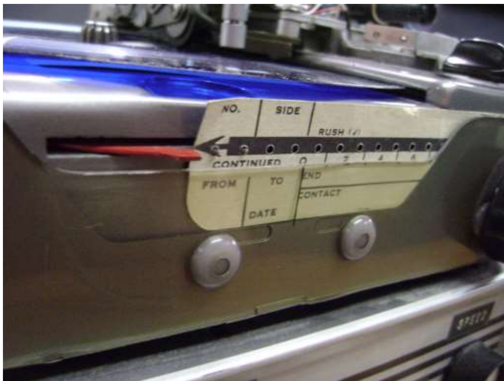
Figure 10: Index strip inserted into the Audograph machine. Photograph by Heather Adkins. Gray Audograph is property of the Tennessee State Library and Archives in Nashville, TN.
