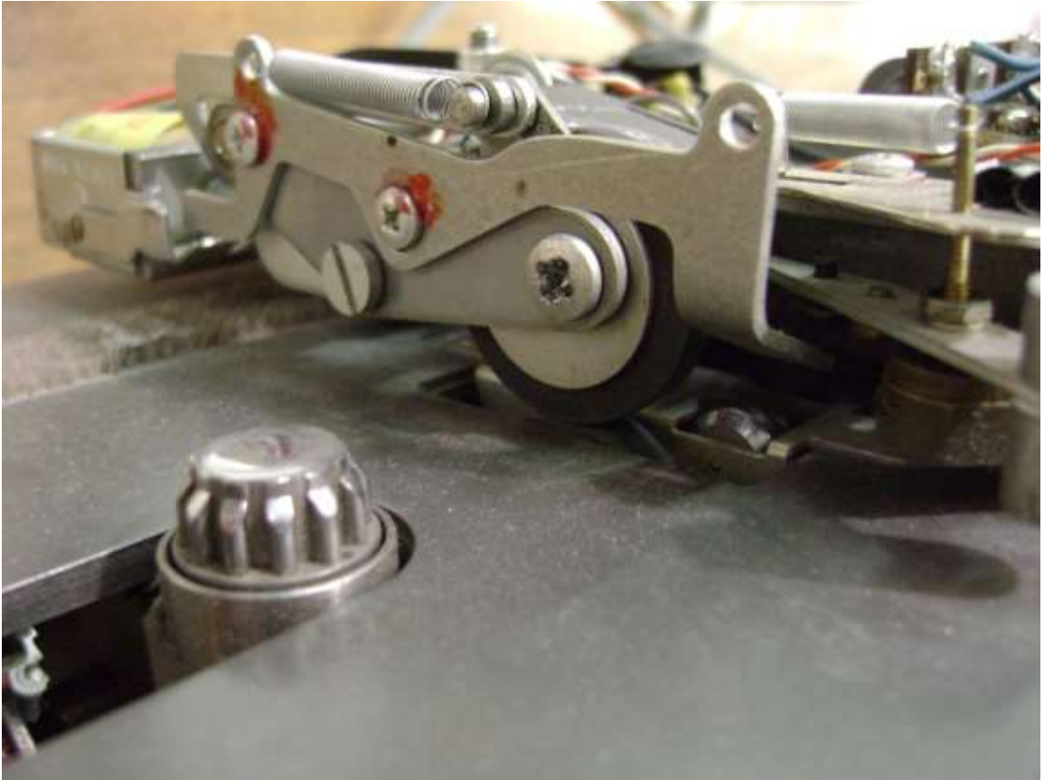
Figure 16: Close up of the star-shaped spindle and pucks. The stylus is hidden on the other side of the pucks. Photograph by Heather Adkins. Gray Audograph is property of the Tennessee State Library and Archives, Nashville, TN.
