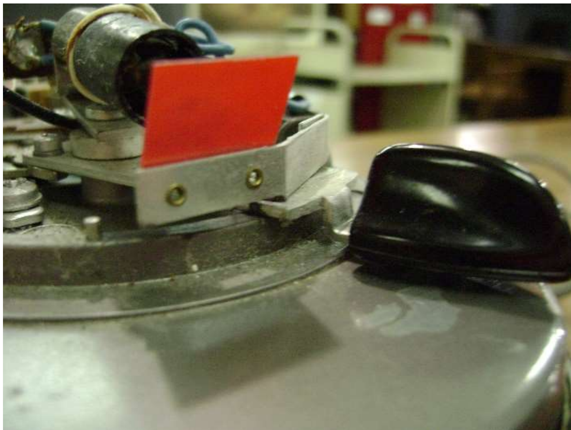
Figure 3: Control switch for recording and playback. Photograph by Heather Adkins. Gray Audograph is property of the Tennessee State Library and Archives, Nashville, TN.
