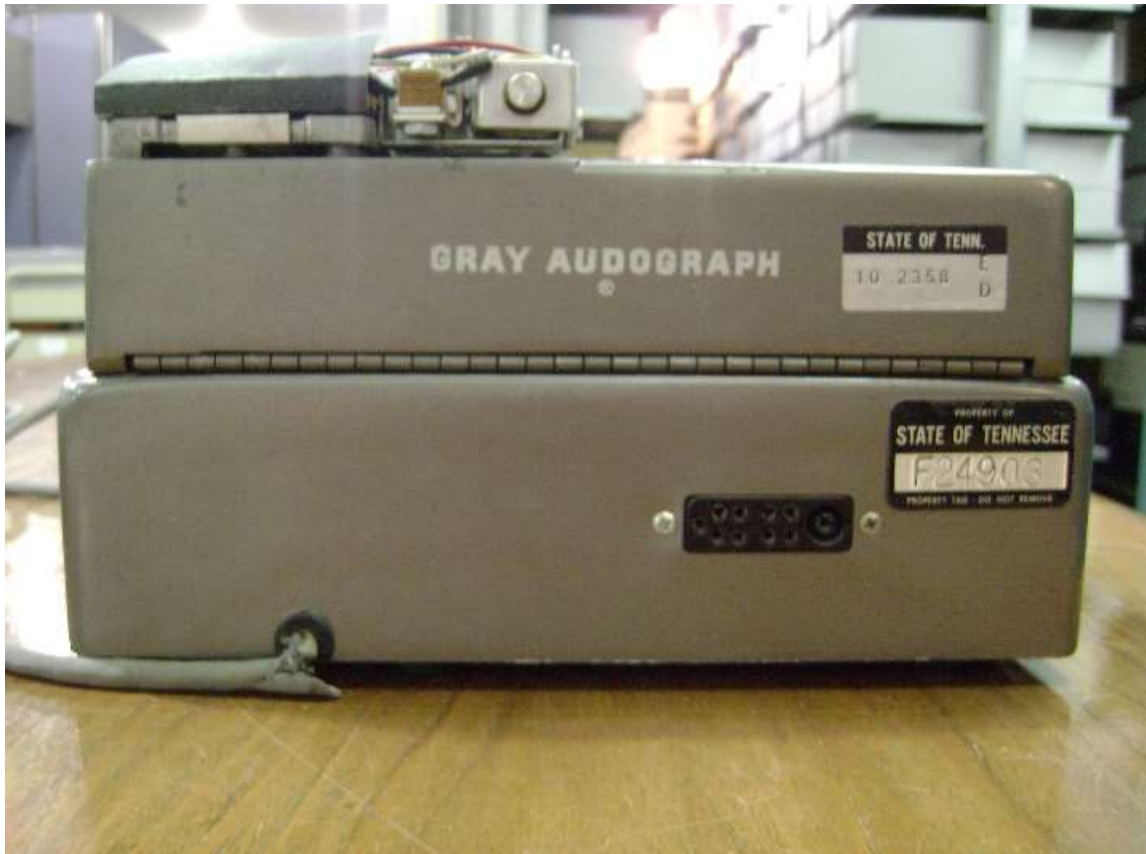
Figure 2: Side of the Audograph featuring the typewriter or foot controller port. Photograph by Heather Adkins. Gray Audograph is property of the Tennessee State Library and Archives, Nashville, TN.
