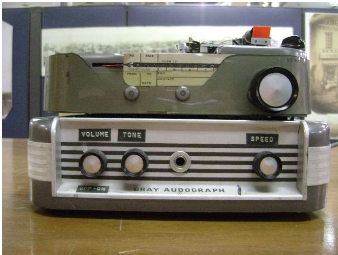
Figure 4: Front of the Audograph featuring the volume, tone, and speed controls. Photograph by Heather Adkins. Gray Audograph is property of the Tennessee State Library and Archives, Nashville, TN.
