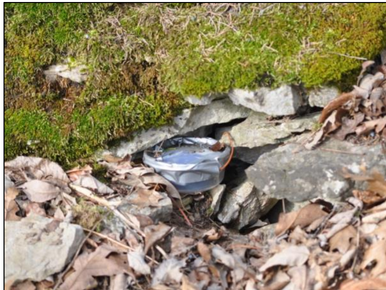
Figure 1: A = Environmental temperatures (soil, air, and den cavities) were measured using single-channel thermocouple wire and data loggers (LOGiT®) housed in water-tight containers; B = Data logger in situ at hibernaculum den cavity (~2 m depth).
