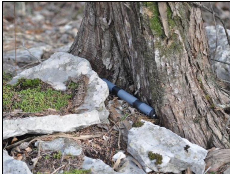
Figure 2: A = Operative snake models were created from 20 cm copper pipes painted grey with two black bands. Rubber stoppers with golf tees were placed on each end to keep the iButton® in the center of the model; B = Operative snake model in situ placed around the denning area to estimate potential thermal minimum and maximum temperatures for snakes on the surface.
