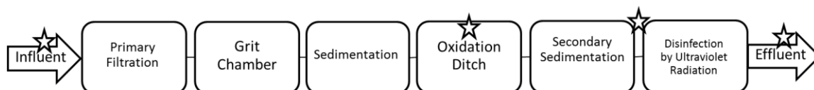
Figure 1. A schematic overview of an activated sludge wastewater treatment plant. Stars represent points along the process where water samples were collected for analysis of estrogenic activity and estrogenic compound concentration.
