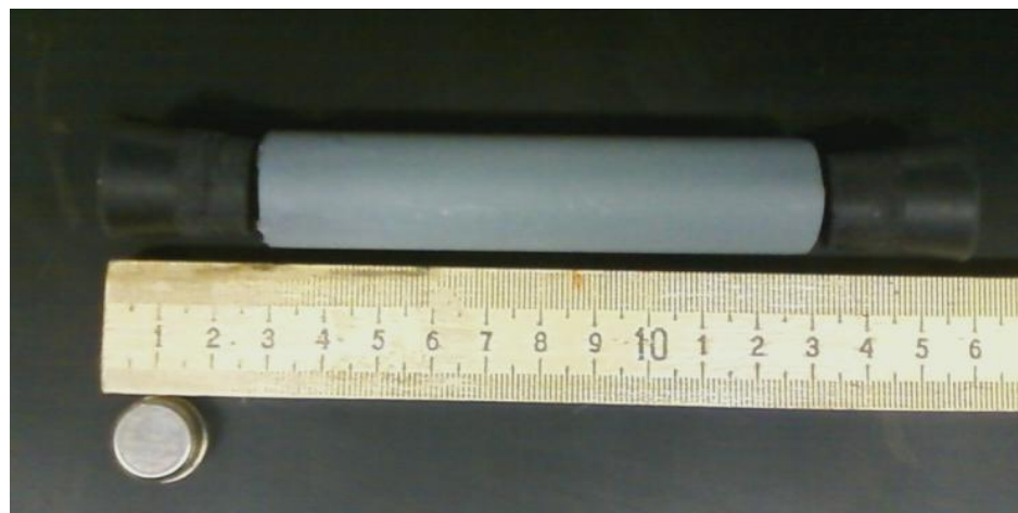
Fig. 2. Operative snake model. Each model contained an iButton® (bottom left).
