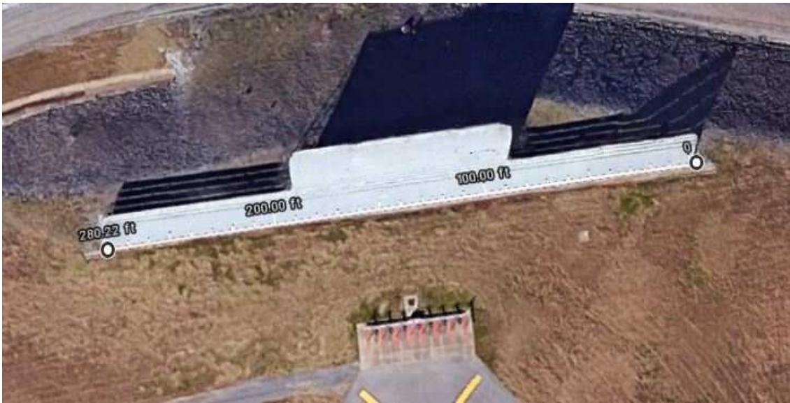
Figure 7. Length of the JBD at the end of runway 13.
