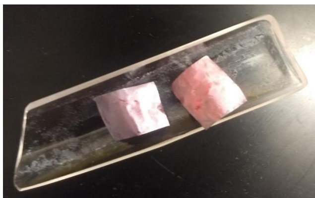
Figure 16. Optical image of Barium Titanate sintered samples in the crucible
