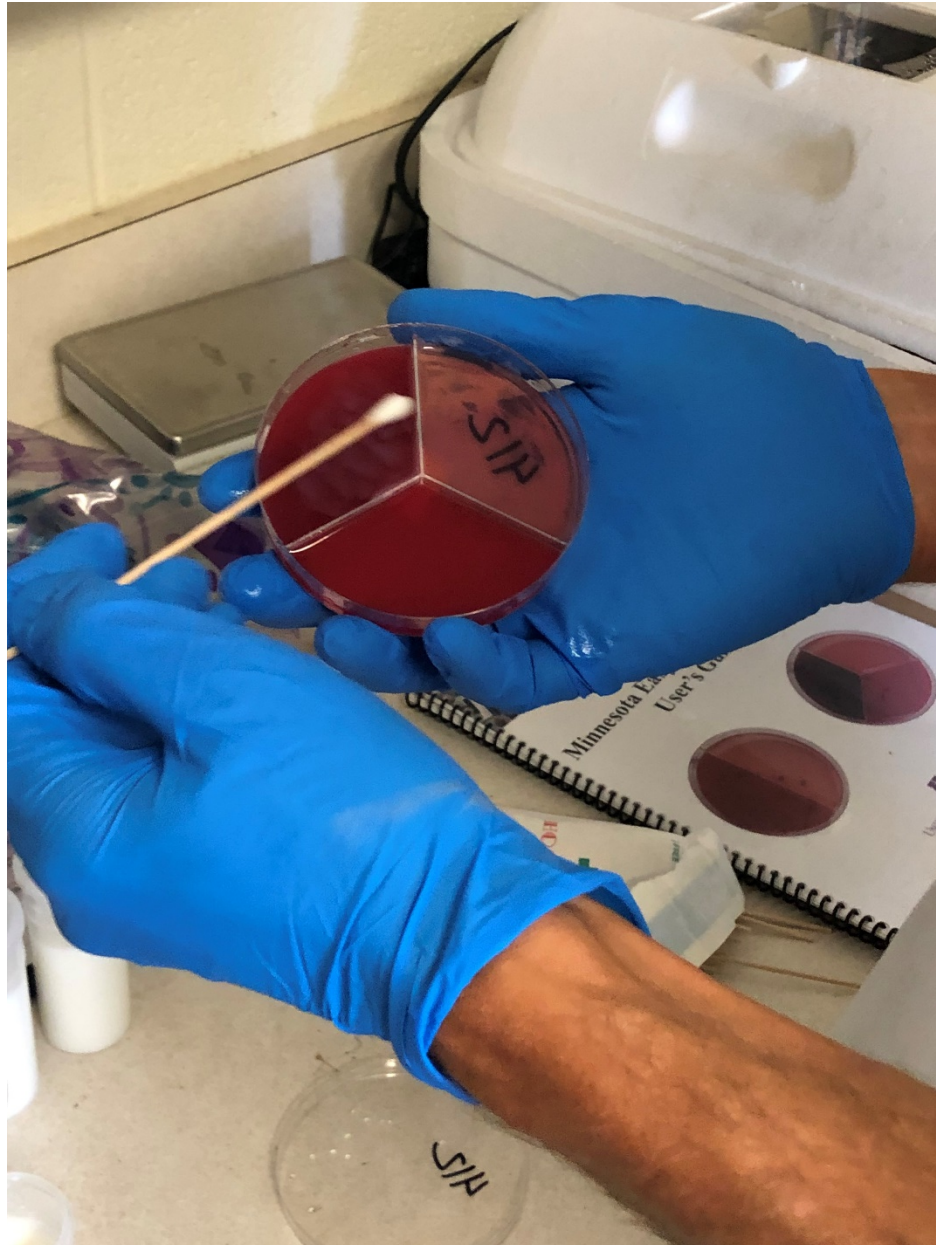
Figure 12. Plating milk samples on a tri-plate culture medium using a sterile swab. The deep red section (top left) is the Focus media, the scarlet section (bottom) is the Factor media, and the pink section (top right) is the MacConkey media. Growth on the Focus and Factor media indicate gram-positive bacterial growth; growth on the MacConkey media indicates gram-negative bacterial growth.
