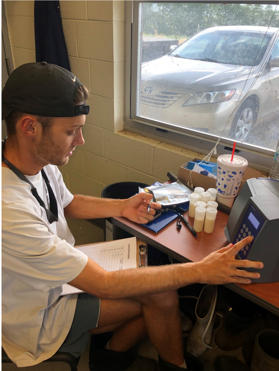
Figure 11. Determining and recording the somatic cell count of each milk sample using the DeLaval Somatic Cell Counter.
