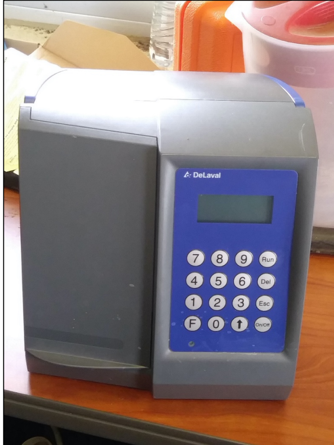
Figure 2. The DeLaval Cell Counter used for on-site somatic cell counts.
