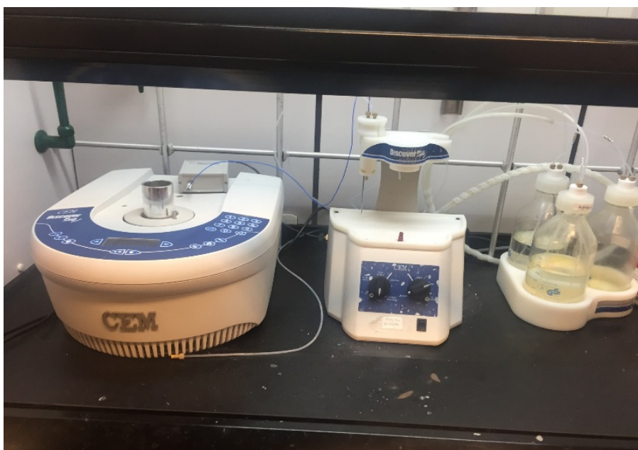
Figure 2. CEM Discover bio manual microwave peptide synthesizer
