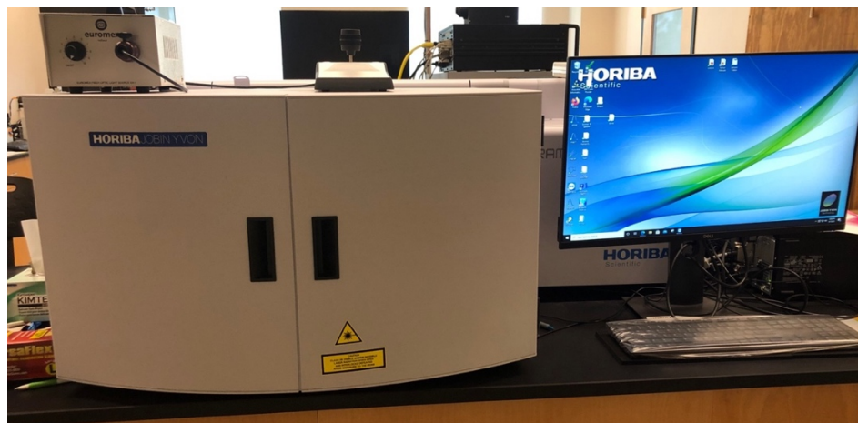
Figure 10. LabRAM HR Evolution confocal Raman microscope with 532 nm excitation laser
