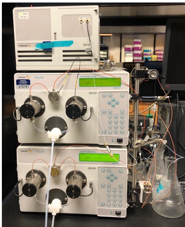
Figure 7. Varian Prepstar SD-1 with Supelco Ascentis C18 column
