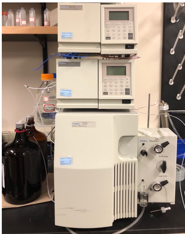
Figure 6. Waters 1525 Binary HPLC pump with Waters 2489 UV/Visible detector
