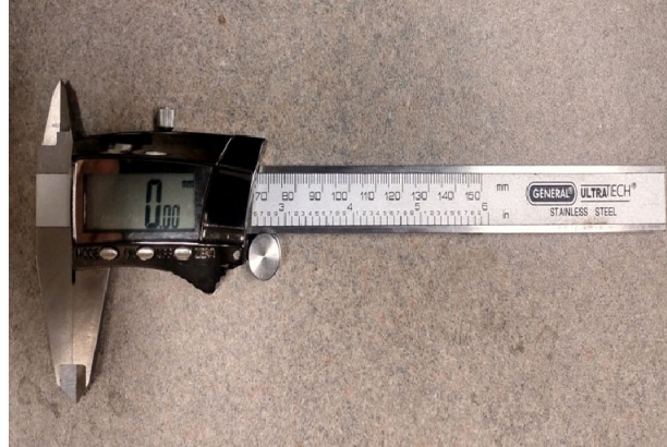
Figure 3. General Tool 6” Steel Digital Caliper 147. Manufactured by Penn Tool Co., Inc located at 1776 Springfield Avenue Maplewood, NJ 07040. This is the digital caliper used to record measurements throughout the study on both the control and experimental groups. Measurements were taken in millimeters.
