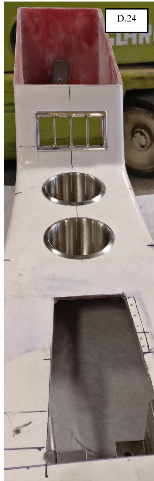
D.23 & D.24 The center console with all holes cut and brackets mounted, before fiberglass work
