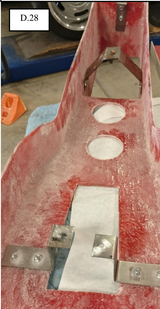
D.27 & D.28 Console mounts before fiberglass work
