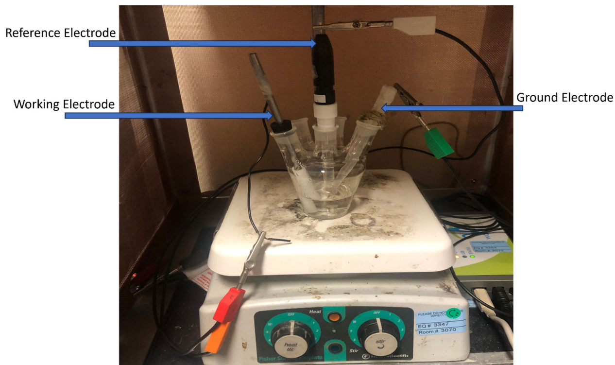
Figure 5: Experimental setup for cyclic voltammetry
