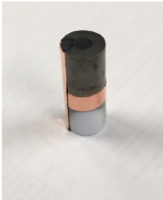
Figure 6: GCE modified with CuO/COOH-MWNT composite, sputter-coated with Au and Pd, and modified with copper tape for SEM and EDX analysis
