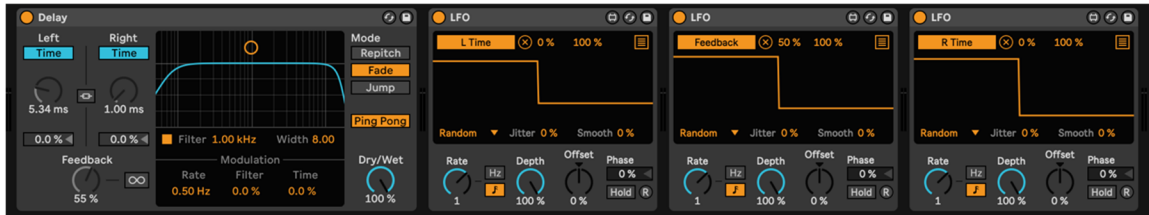
Fig. 7. LFOs randomly modulating the delay’s feedback and time parameters
