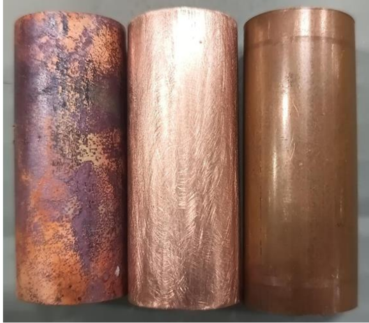
Figure 11: From right to left, the image above first shows the cathode style that will be used for the majority of the batteries tested, the next, middle cathode, has been sanded down to allow the cathodes to be annealed, and the left most cathode shown is one that has been annealed using propane as a heating source.
