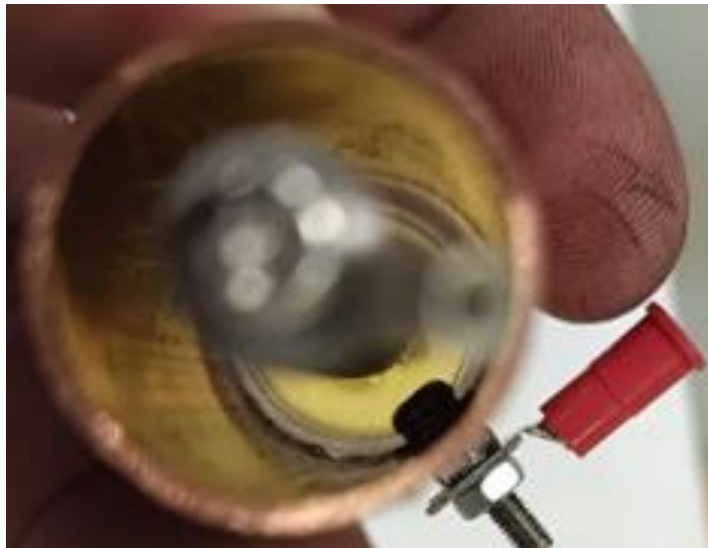
Figure 8: Here is the same test fabrication model but shown from a top-down view. Note, special attention was taken to prevent the bolt head from bridging the cavity between the magnesium anode and the copper cathode and causing a short in the battery.
