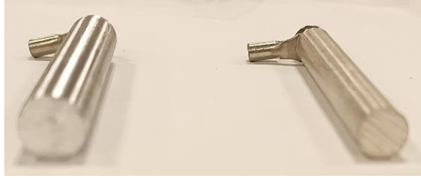
Figure 4: Showcased above are the anode variants used during testing. The anode on the right is a 99.9% pure magnesium rod that is 8mm in diameter and the rod on the left is composed of the same purity but is 9.5mm in diameter.
