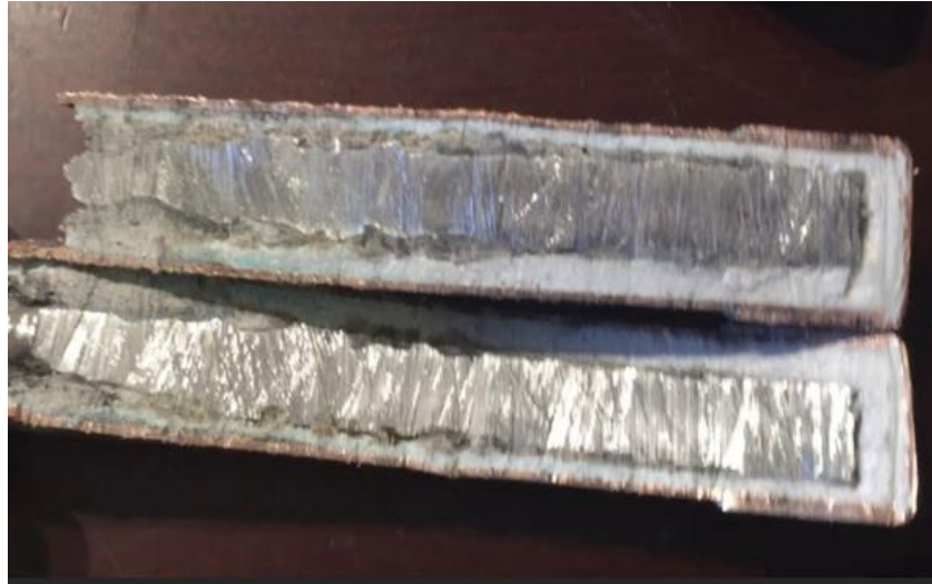
Figure 16: Above shows a cell made in a very similar manner to the cells constructed for this experiment. The cell shown has been bisected down the middle in an attempt to observe the degradation of the cell. This specific cell was used in conjunction with other crystal-cell batteries to operate a motor that started spinning in December 2011 and was observed to run for 1429 days. Source: (Lasersaber, 2015).
