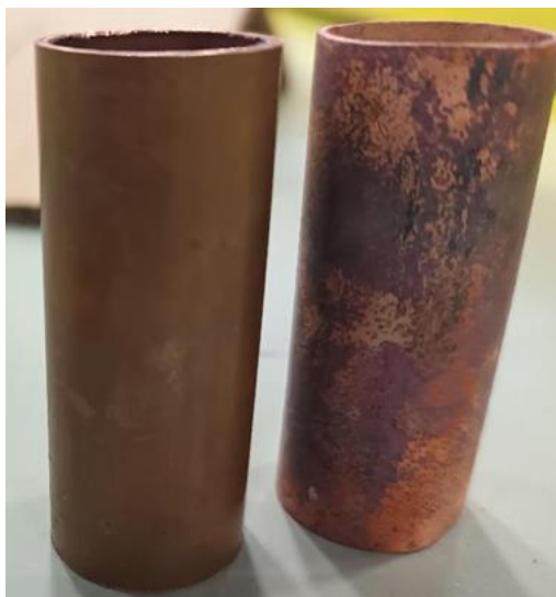
Figure 14: Above shows the physical difference between the cathodes that were annealed using the propane heating and the non-annealed cathodes.
