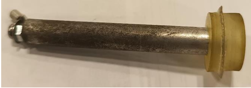
Figure 6: Shows the test anode used to assure that the parts were fabricated correctly. Note the discoloration observed on the anodes surface. The isolation in air-tight plastic bags prevented this from occurring to the anodes that were used in this experiment.
