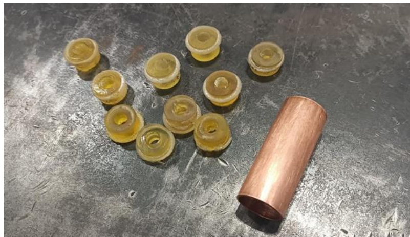
Figure 5: Above shows the polyurethane grommets used next to the copper cathode that they were fitted into.
