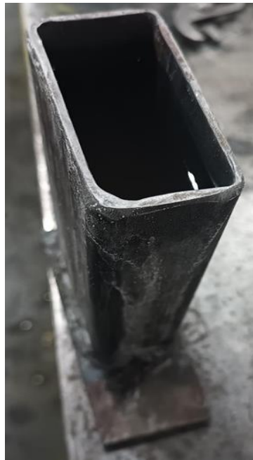
Figure 9: Above is the quench tank that was fabricated so that the cathodes could be quenched using distilled water and sodium tetraborate to create a super saturated solution.
