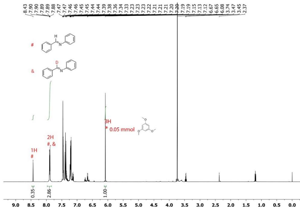
Figure 2.2  $^1\text{H}$  NMR (500 MHz,  $\text{CDCl}_3$ ) of the coupling reaction of benzyl alcohol- $\alpha,\alpha\text{-d}_2$  and aniline to N-benzylideneaniline.
