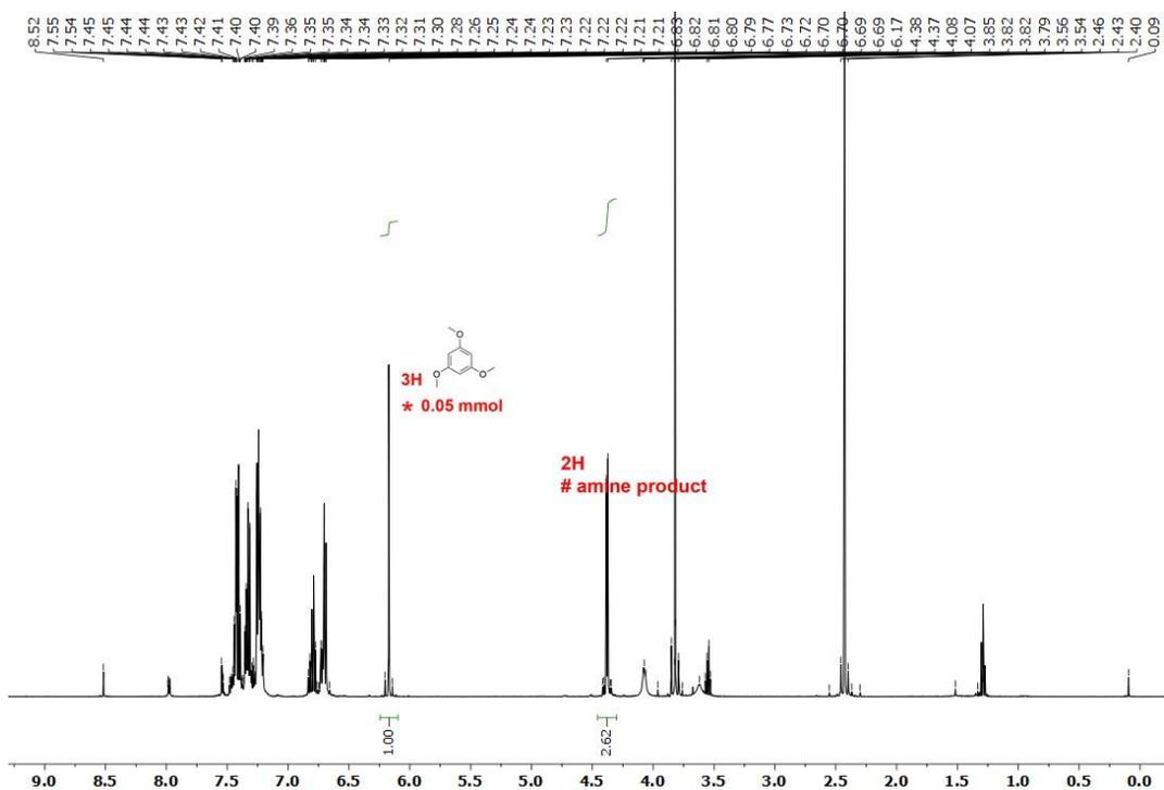
Figure 2.10  $^1\text{H}$  NMR (500 MHz,  $\text{CDCl}_3$ ) of the reaction mixture of amine synthesis by II and  $\text{KO}^t\text{Bu}$ .
