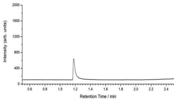
Figure 4.2 H<sub>2</sub> detection by GC chromatography.
