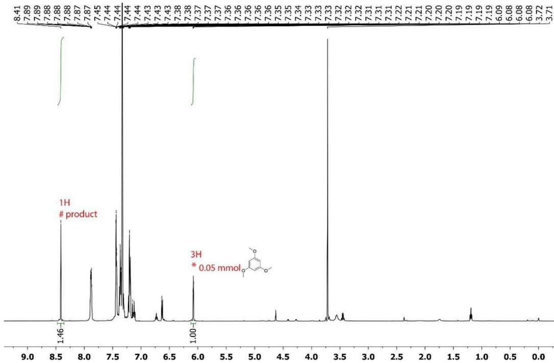
Figure 2.5  $^1\text{H}$  NMR (500 MHz,  $\text{CDCl}_3$ ) of the reaction mixture of 3a.
