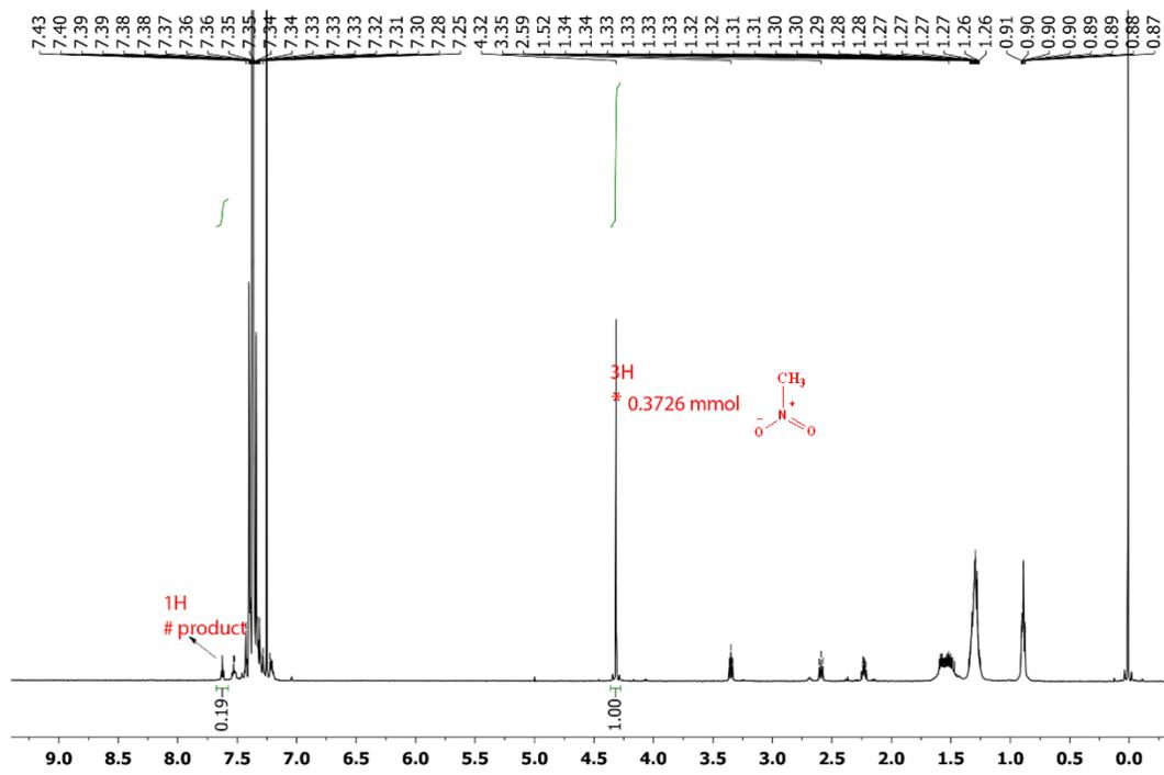
Figure 2.45  $^1\text{H}$  NMR (500 MHz,  $\text{CDCl}_3$ ) of the reaction mixture of 3ab.
