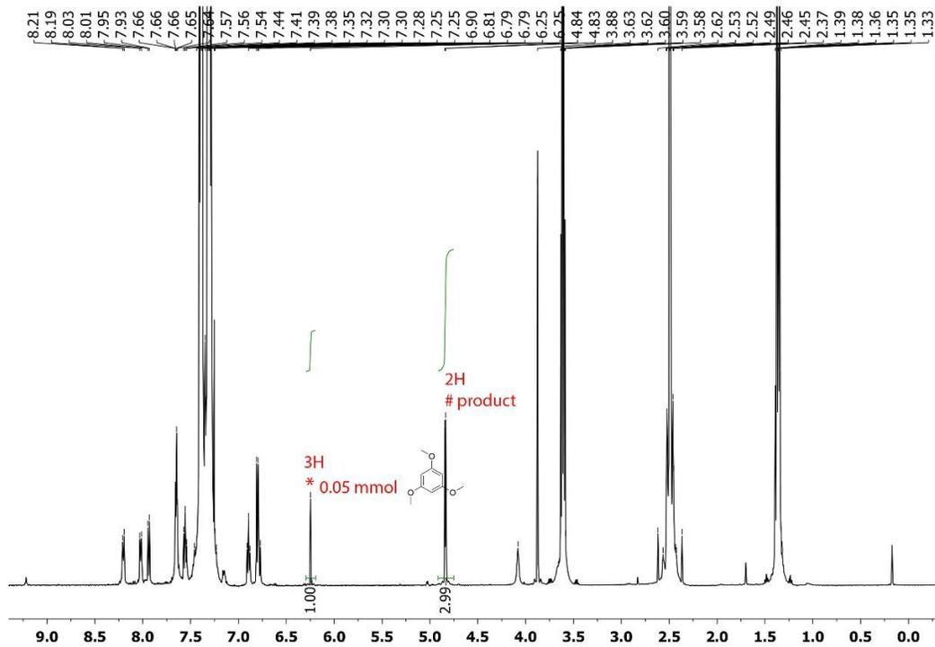
Figure 2.64  $^1\text{H}$  NMR (500 MHz,  $\text{CDCl}_3$ ) of the reaction mixture of 4t.
