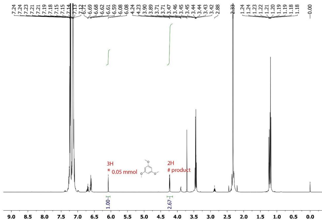
Figure 2.50  $^1\text{H}$  NMR (500 MHz,  $\text{CDCl}_3$ ) of the reaction mixture of 4e.
