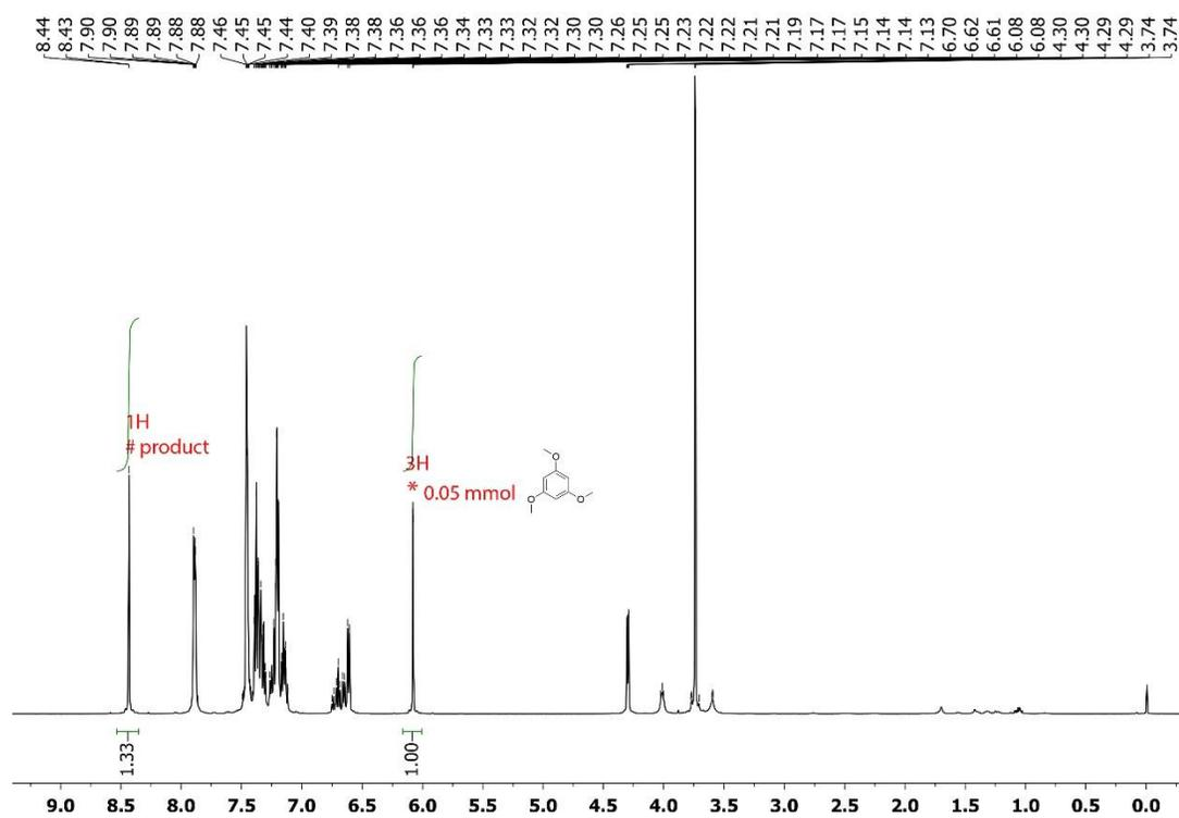
Figure 2.15  $^1\text{H}$  NMR (500 MHz,  $\text{CDCl}_3$ ) of the reaction mixture of imine synthesis by V and  $\text{KO}^t\text{Bu}$ .
