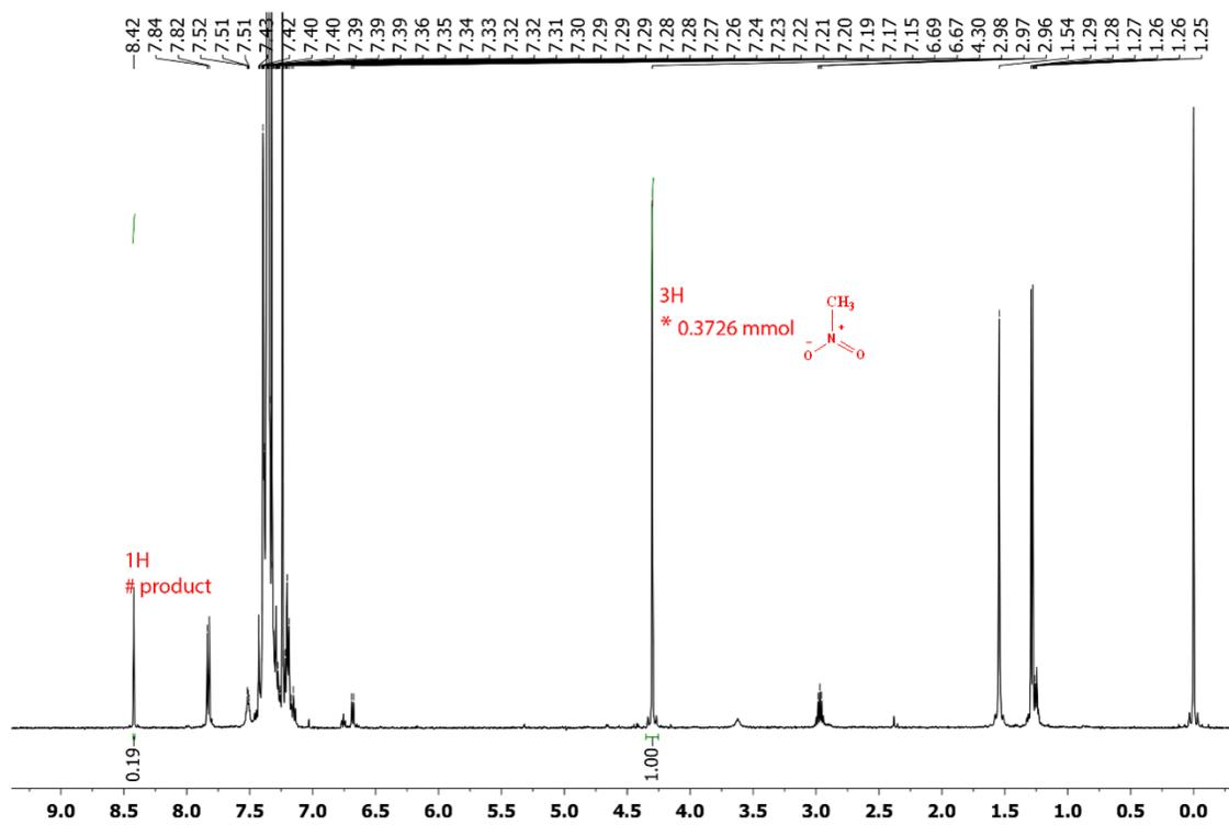
Figure 2.22  $^1\text{H}$  NMR (500 MHz,  $\text{CDCl}_3$ ) of the reaction mixture of 3e.
