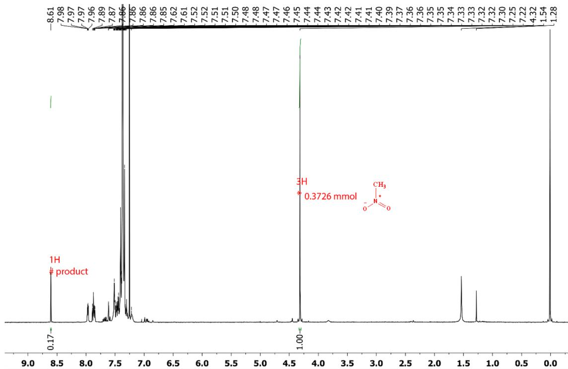
Figure 2.39  $^1\text{H}$  NMR (500 MHz,  $\text{CDCl}_3$ ) of the reaction mixture of 3v.
