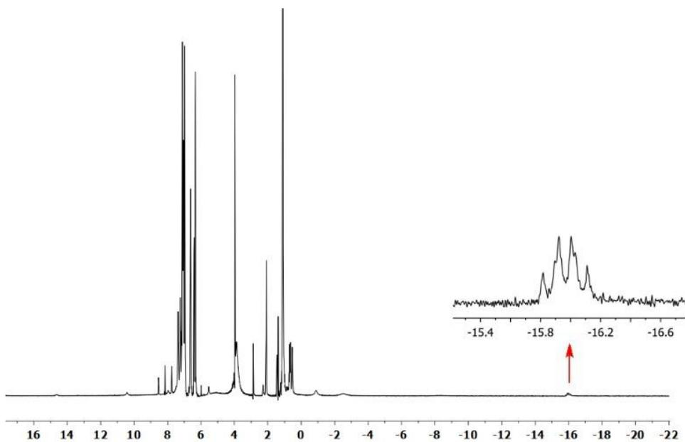
Figure 2.3  $^1\text{H}$  NMR (500 MHz, toluene- $d_8$ ) of the reaction mixture of benzyl alcohol and aniline coupling to N-benzylaniline. A cobalt hydride species was observed at  $-15.99$  ppm.
