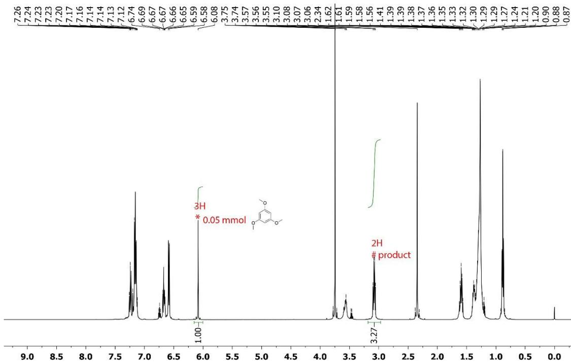
Figure 2.71  $^1\text{H}$  NMR (500 MHz,  $\text{CDCl}_3$ ) of the reaction mixture of 4af.
