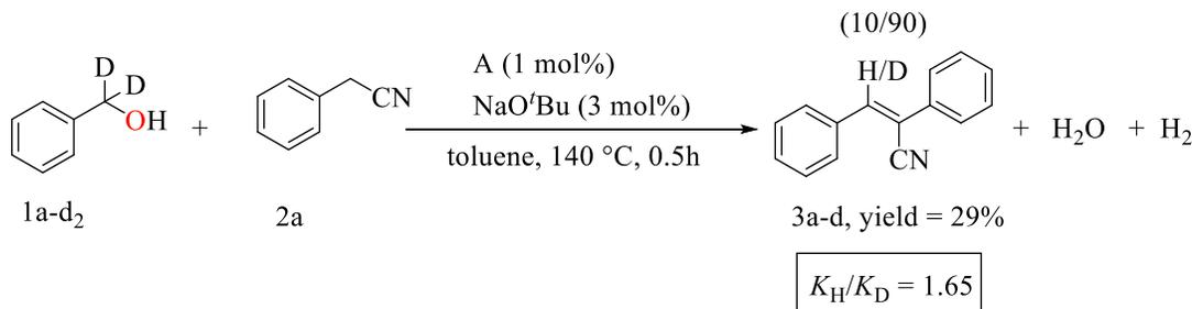
Scheme 4.3 Deuterium labeling experiment using 1a- d<sub>2</sub>
