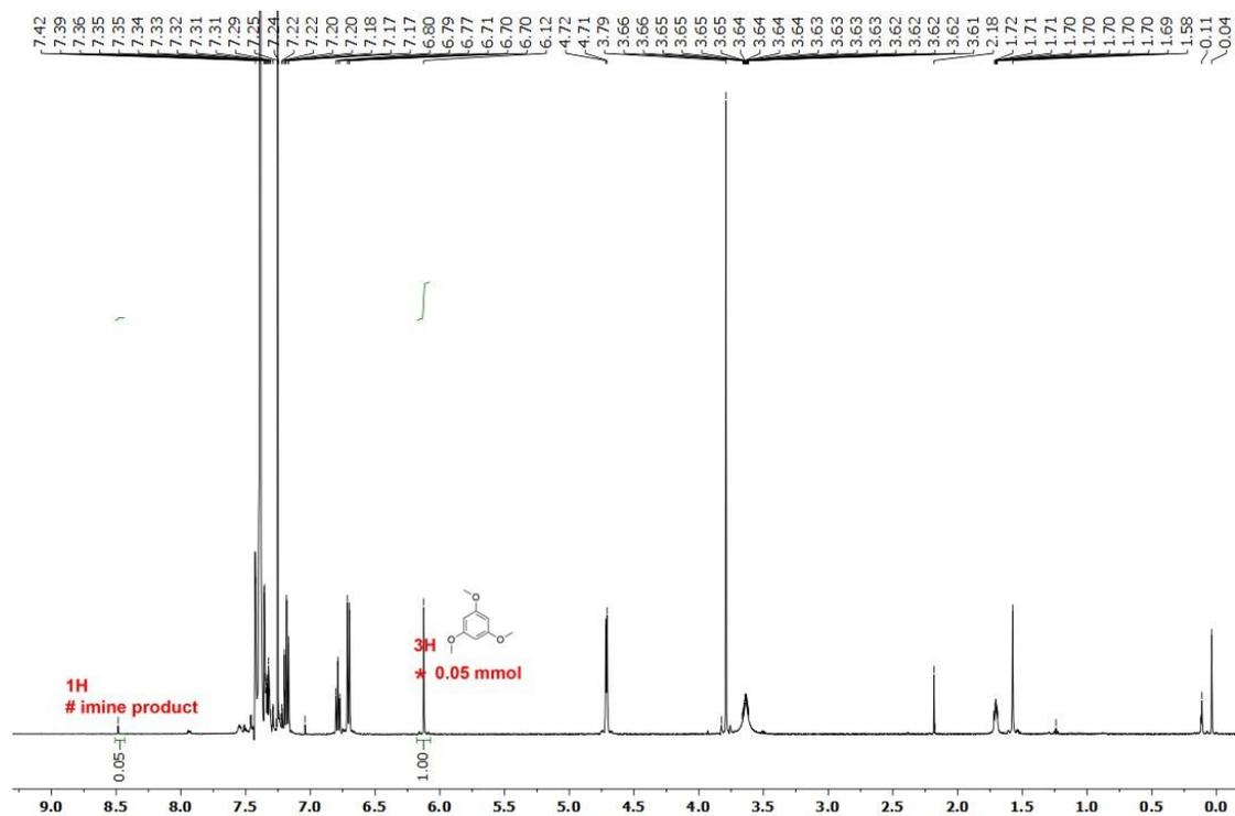
Figure 2.17  $^1\text{H}$  NMR (500 MHz,  $\text{CDCl}_3$ ) of the reaction mixture of imine synthesis by VI and KO<sup>t</sup>Bu.
