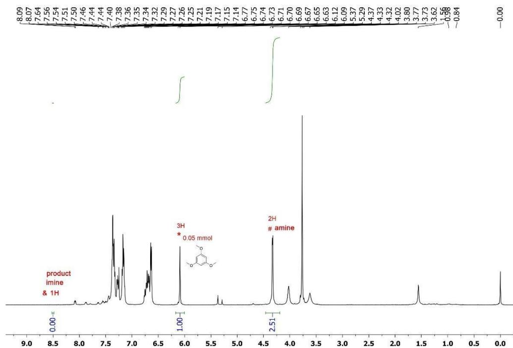
Figure 2.13  $^1\text{H}$  NMR (500 MHz,  $\text{CDCl}_3$ ) of the reaction mixture of imine synthesis by IV and  $\text{KO}^t\text{Bu}$ .
