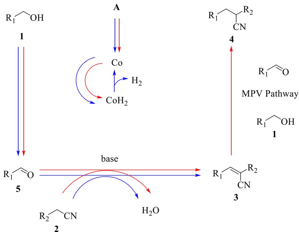
Scheme 4.5 Proposed mechanism ( $\alpha$ -Olefination in Blue and  $\alpha$ -alkylation in Red)
