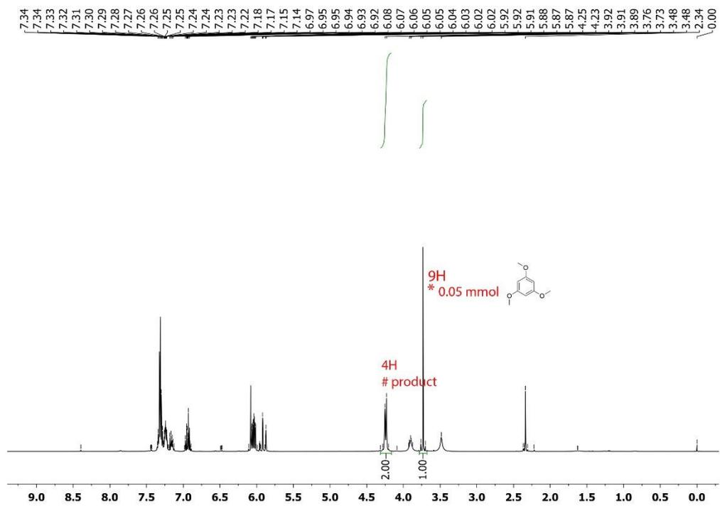
Figure 2.75  $^1\text{H}$  NMR (500 MHz,  $\text{CDCl}_3$ ) of the reaction mixture of 4aj.
