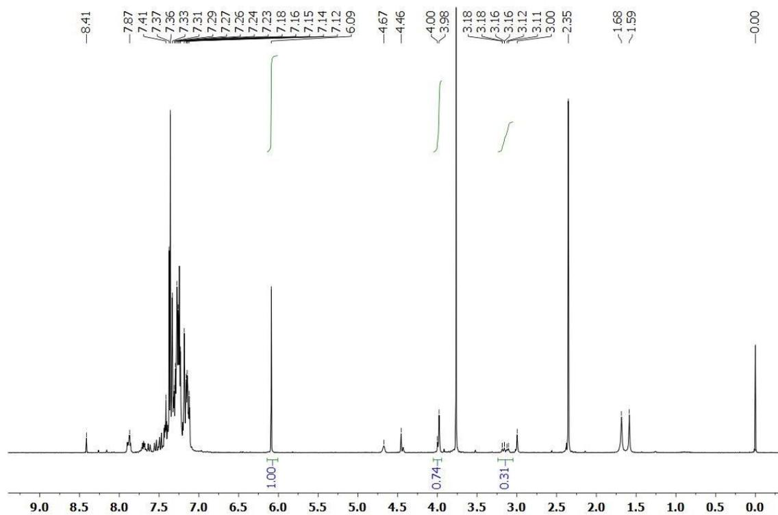
Figure 3.71 <sup>1</sup>H NMR Spectra (CDCl<sub>3</sub>, 500 MHz) of the deuterium labeling experiment for the  $\alpha$ -alkylation of phenylacetonitrile with benzyl alcohol- $\alpha,\alpha$ -d<sub>2</sub>.
