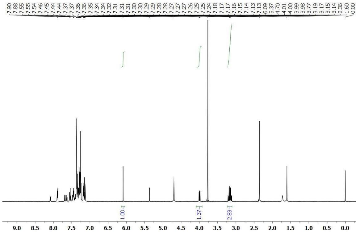
Figure 3.68  $^1\text{H}$  NMR Spectra ( $\text{CDCl}_3$ , 500 MHz) of the deuterium labeling experiment for the 2,3-diphenylacrylonitrile transfer hydrogenation using benzyl alcohol.
