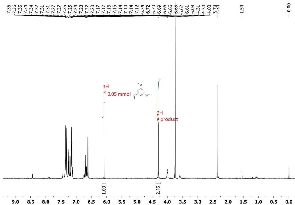
Figure 2.16  $^1\text{H}$  NMR (500 MHz,  $\text{CDCl}_3$ ) of the reaction mixture of amine synthesis by VI and  $\text{KO}^t\text{Bu}$ .
