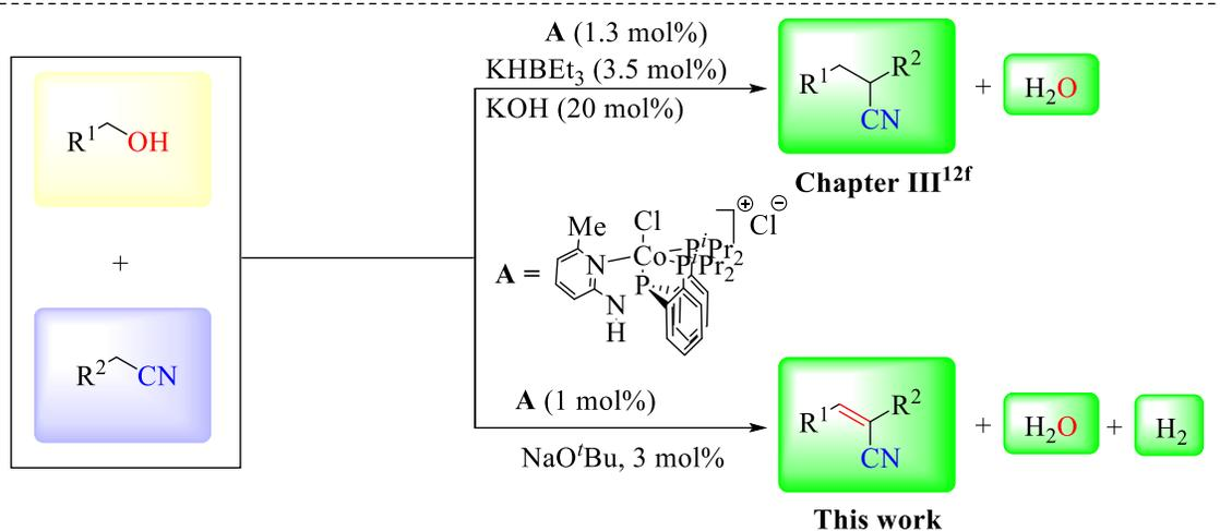
Scheme 4.1 Switchable  $\alpha$ -Alkylation and  $\alpha$ -olefination of Nitriles with Primary Alcohols Catalyzed by Ding's cobalt catalyst
