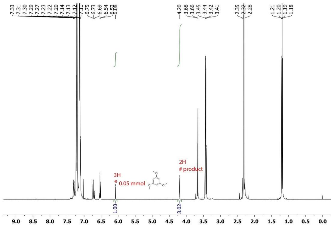
Figure 2.52  $^1\text{H}$  NMR (500 MHz,  $\text{CDCl}_3$ ) of the reaction mixture of 4g.
