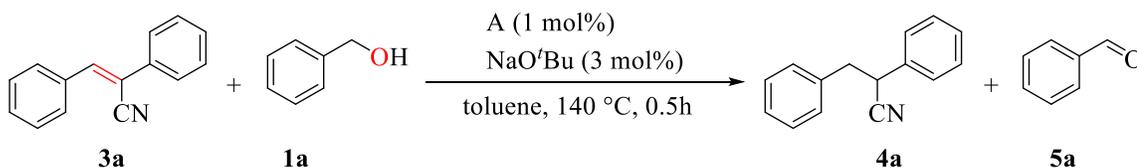
Scheme 4.4. Transfer hydrogenation of 2,3 Diphenylacrylonitrile
