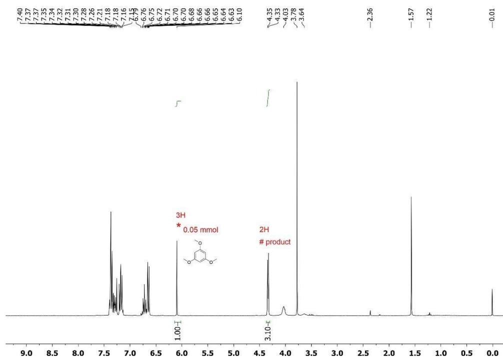
Figure 2.14  $^1\text{H}$  NMR (500 MHz,  $\text{CDCl}_3$ ) of the reaction mixture of amine synthesis by IV and  $\text{KO}^t\text{Bu}$ .
