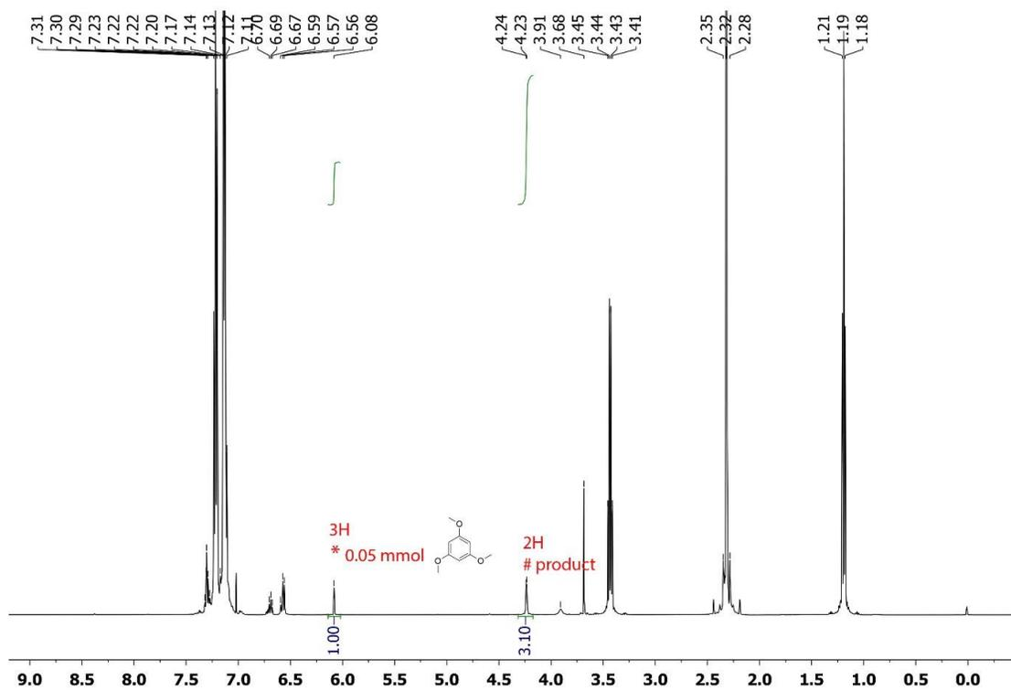
Figure 2.7  $^1\text{H}$  NMR (500 MHz,  $\text{CDCl}_3$ ) of the reaction mixture of 4a.
