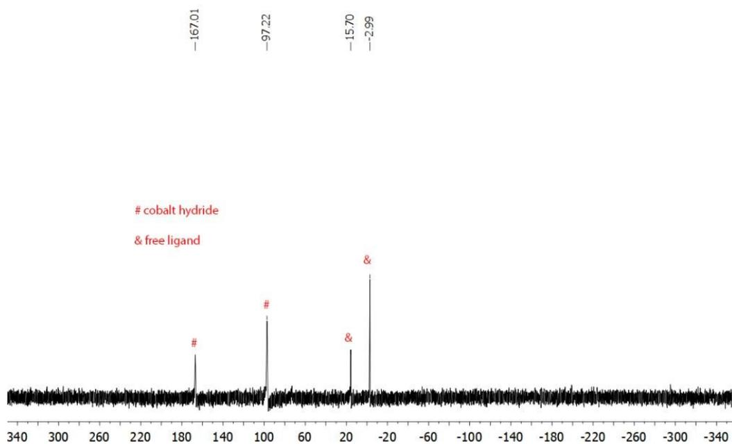
Figure 2.4  $^{31}\text{P}$  NMR (122 MHz, toluene- $d_8$ ) of the reaction mixture of benzyl alcohol and aniline coupling to N-benzylaniline.
