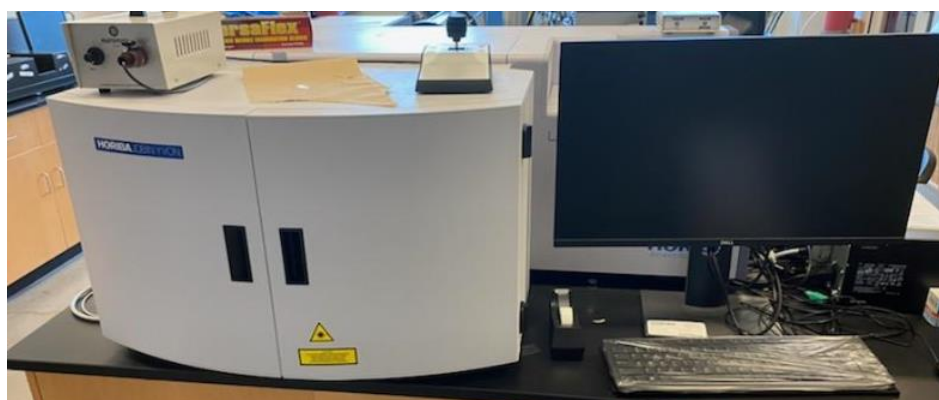
Figure 2.6. Lab Ram HR Evolution confocal Raman microscope.
