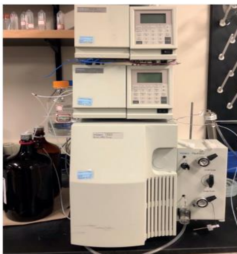
Figure 2.5. HPLC Waters 1525 system.
