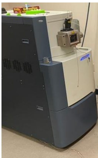
Figure 2.4. Waters Synapt tandem mass spectrometer with time-of-flight configuration.
