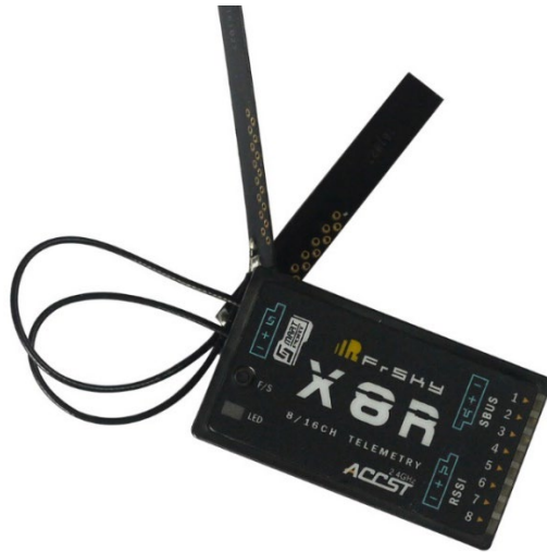
Figure 20. FrSky X8R receiver [29].
