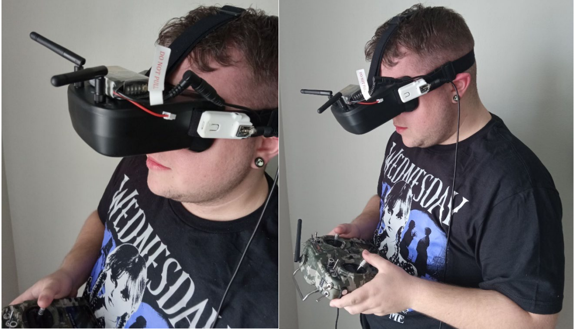
Figure 33. Close view of the head tracker mounted on goggles (left) and the full system being used (right).
