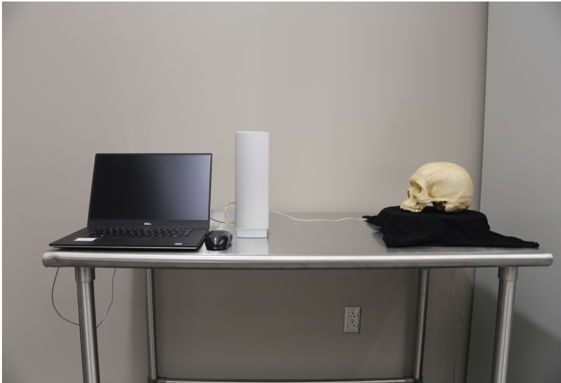
Figure 8: Set-up used for the NextEngine 3-D Laser Scanner.
