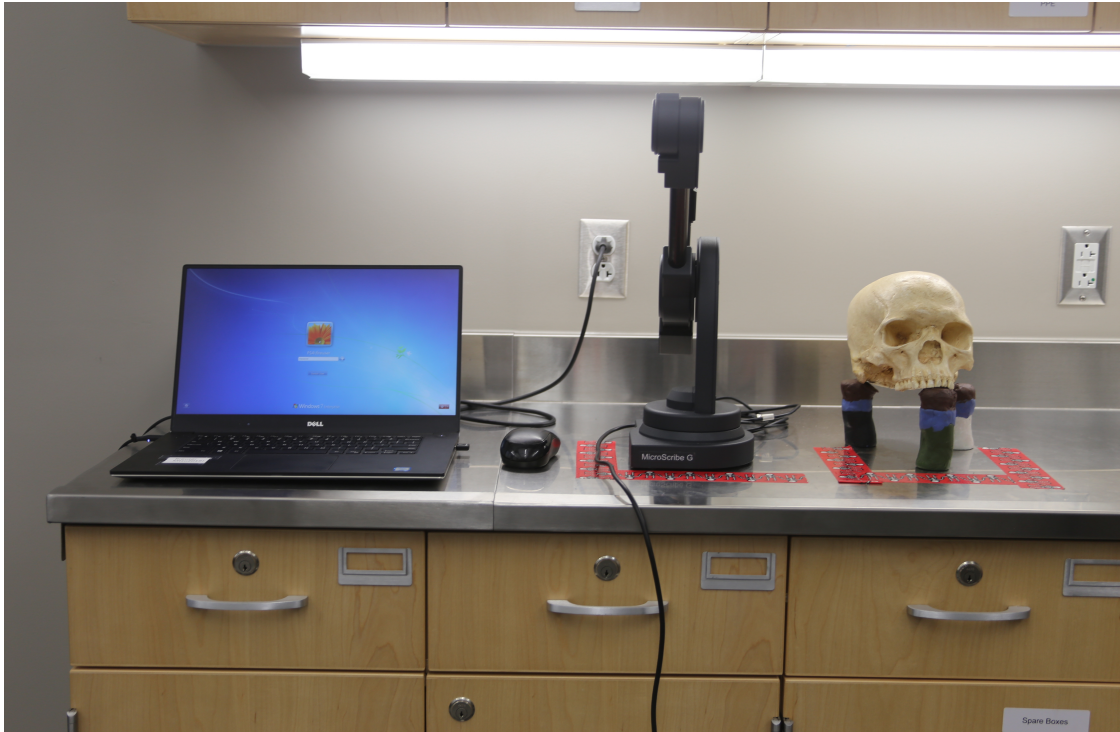
Figure 19: Typical set up of the Microscribe 3-D Digitizer.
