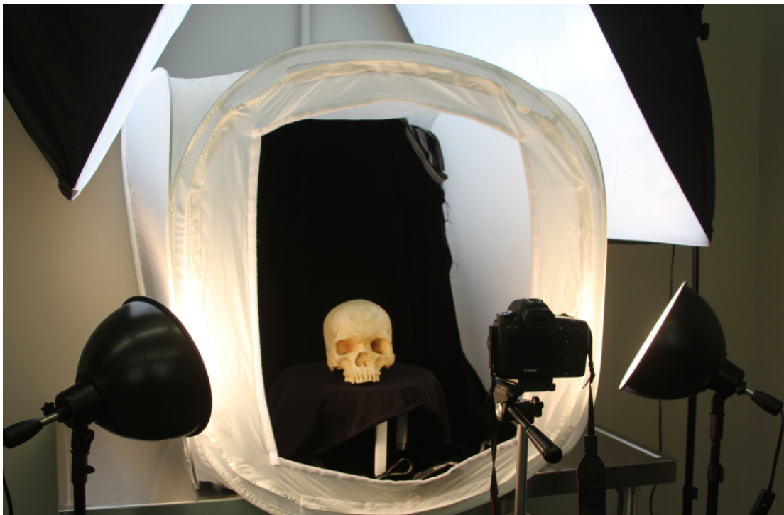
Figure 13: Photogrammetry set up with Individual 2 placed on the rotating turn table. Softbox lights are set up above and to the right and left of the subject. Can lights are set in front of the subject beside the camera.
