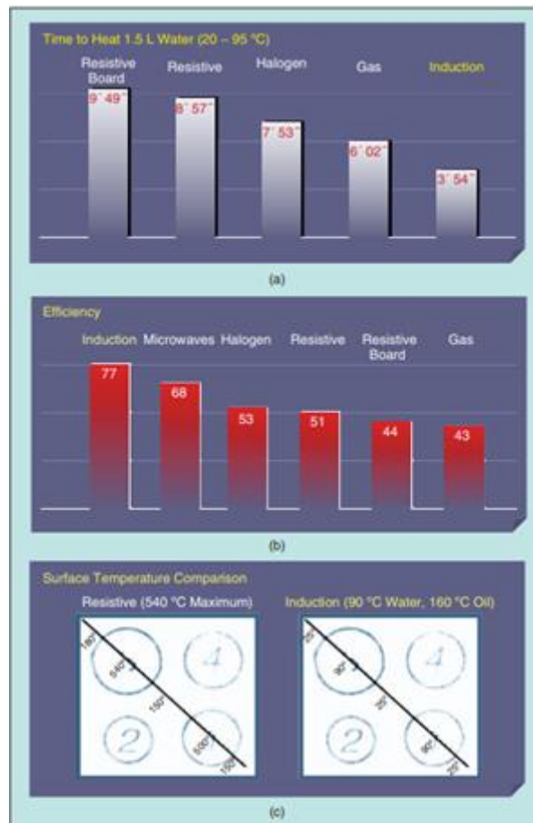
Figure 5: A comparison of domestic heating technologies: (a) heating times, (b) efficiency, and (c) surface temperature [20]
