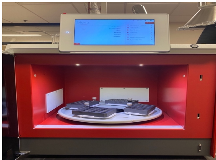
Figure 2.1. Microwave-assisted Extraction Set-Up
