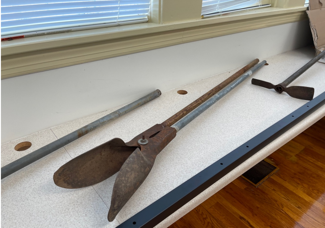
Figure 38. Photo of a post-hole digger at Townsend School. Photo provided by Emily Huffer.
