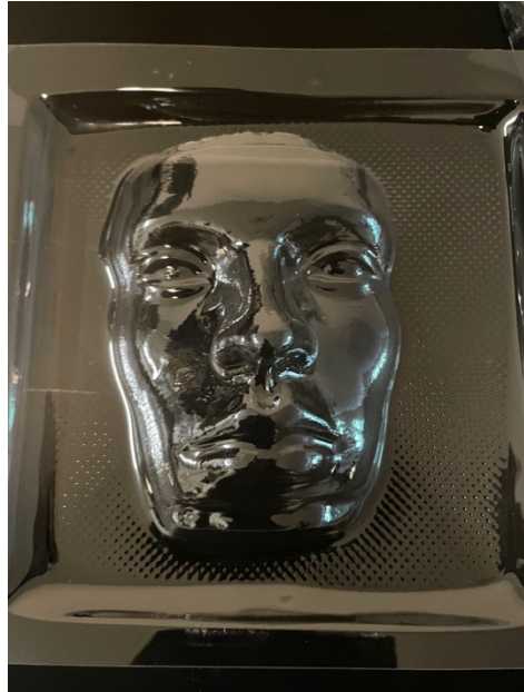
Figure 10: Vacuum formed plastic mask before cutting
