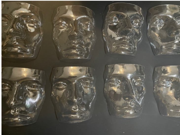
Figure 11: Masks after cutting and hole punching
