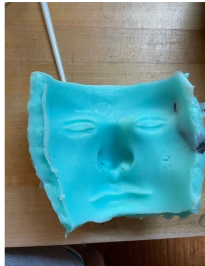
Figure 2: Silicone mold of mannequin face
