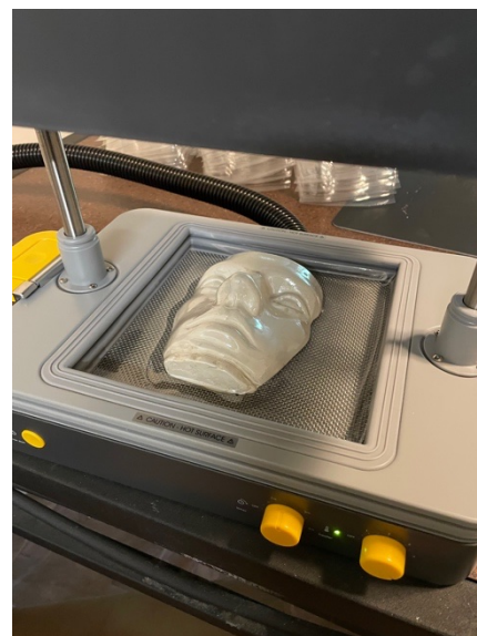
Figure 8: Plastic sheet cooling on plaster mask
