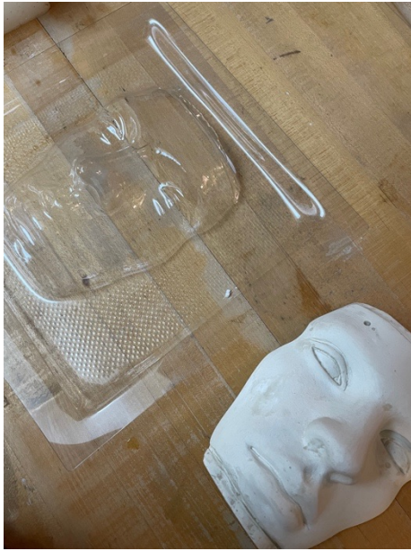
Figure 9: Vacuum formed plastic sheet next to plaster face
