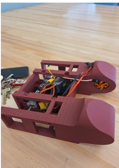
Figure 2.5 – An illustration of a mechatronics system in A regular combat robot (MTSU robotics club, Combat 5, Team robot)
