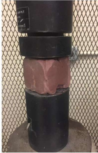
Figure 7: Sulfur concrete cube in the Instron Satec compression machine.
