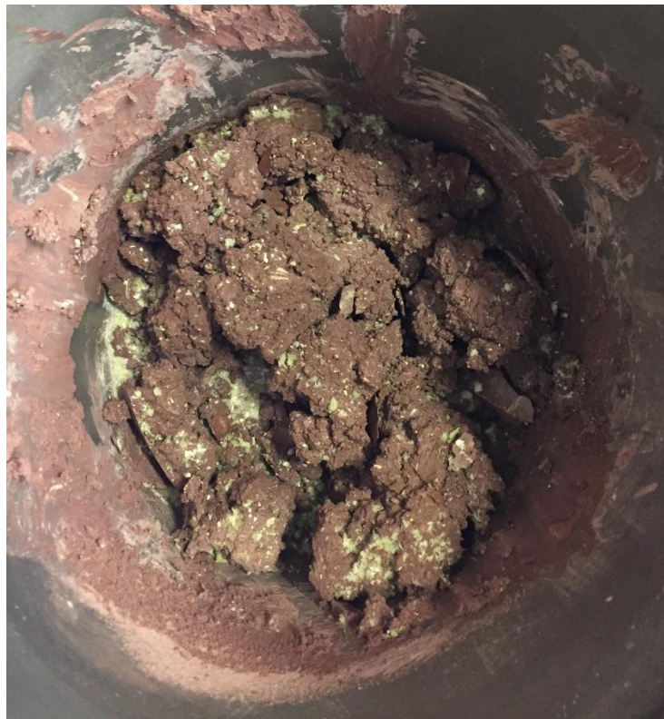
Figure 3: 50/50 Sulfur-soil simulant mixture after 1 ½ hours of heating.
