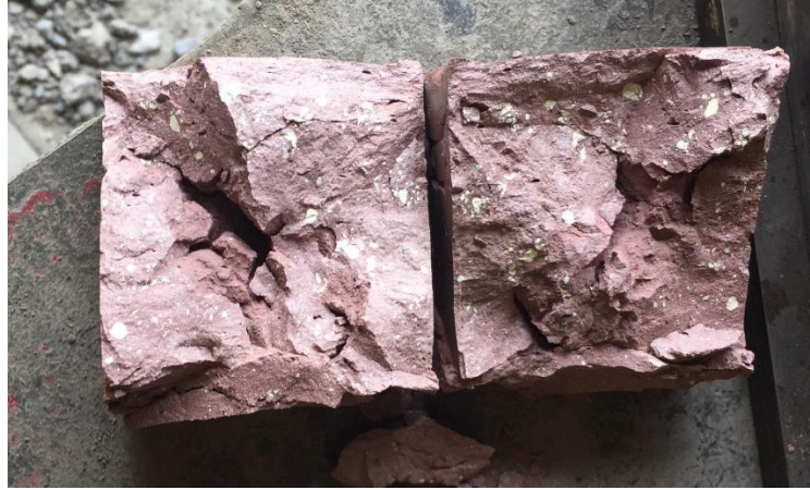
Figure 12: Central void in sulfur concrete cube 1A.
