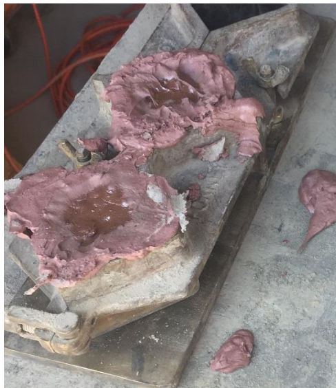
Figure 6: Center subsidence of sulfur concrete in cube forms.
