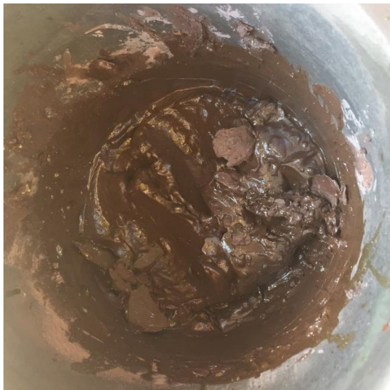
Figure 4: Recreated soil simulant and sulfur (60%).
