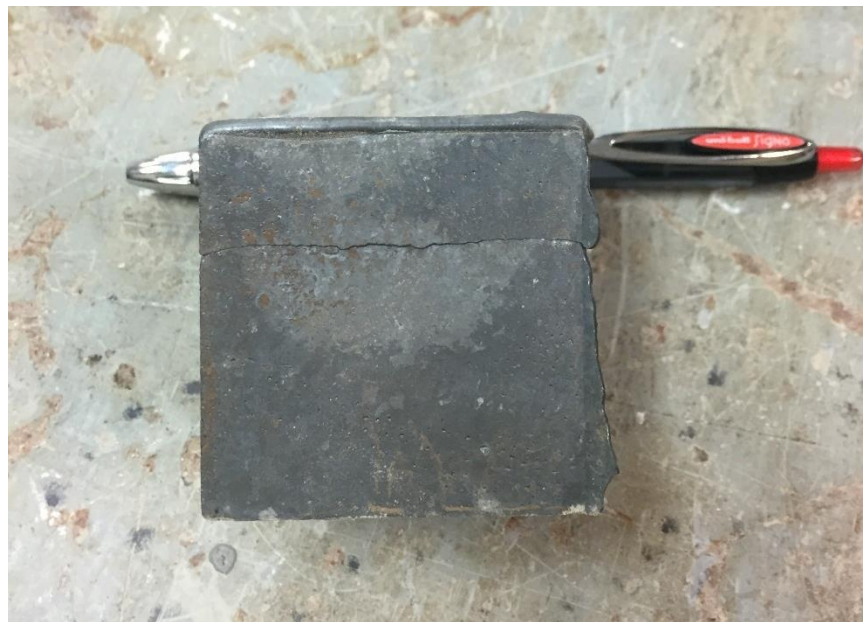
Figure 5: Cold joint shown in a practice cube made of sulfur capping compound.
