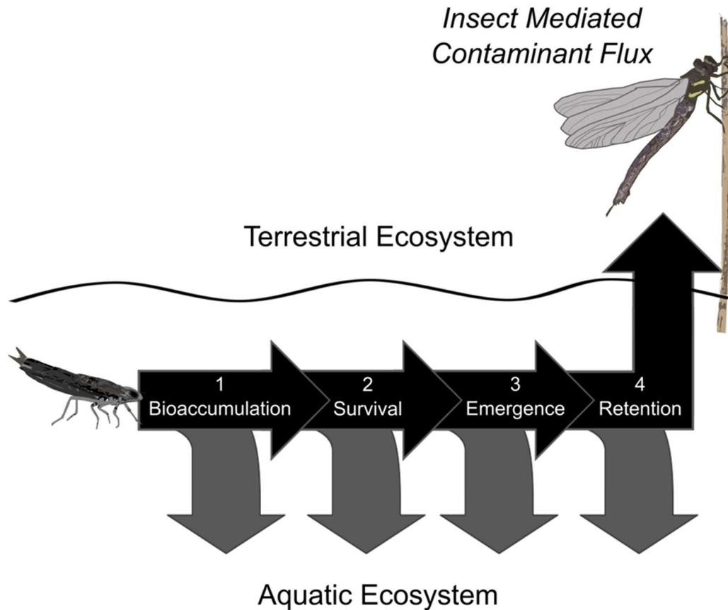
Figure 2. The Riparian Impact Test. A stepwise decision tool to assess if insect-mediated contaminant flux should be considered in an ecological risk assessment. Each numbered arrow represents a condition of the test. If the condition is not met, then the contaminant is retained in the aquatic ecosystem (gray arrows).
