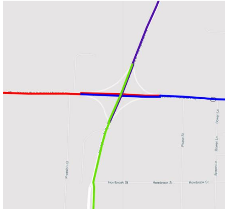
FIGURE 3-5 COMPLEX CROSS-INTERSECTION FORMED USING EIGHT PAIRS OF SEGMENTS AT TN-104 AND US-51 BYP.
