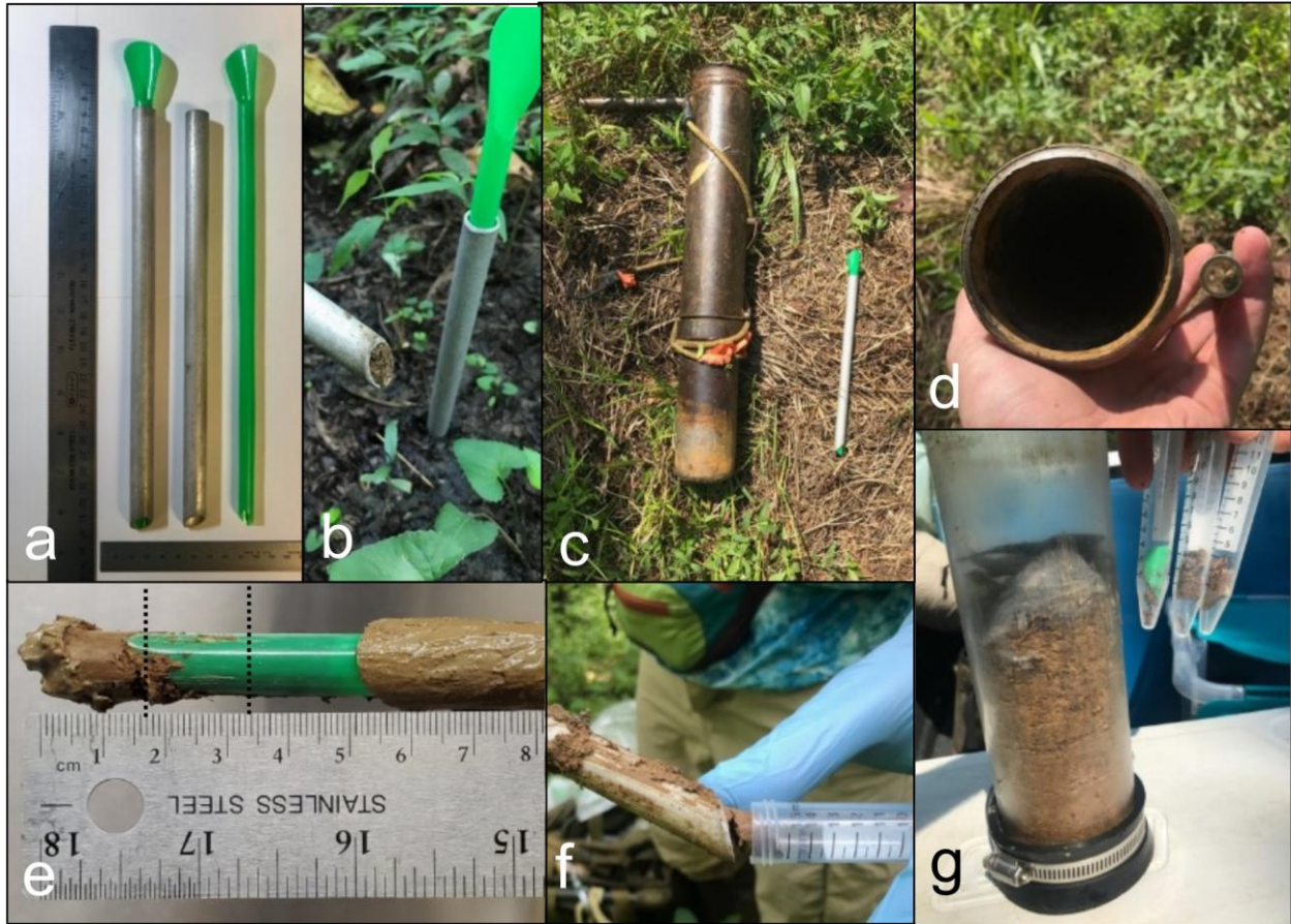
Figure 2. Field sampling methodology. Microbial soil sampling rods consist of an aluminum rod exterior with an VWR spatula inside (a). Sterilized sampling rods are used to collect soil samples in the field (b). Soil sampling rods are compared to incubation core collection devices (c, d). Soil sampling rods collect a consistent 5cm soil sample (e) which is aseptically partitioned in the field (f) into top, middle and bottom partitions (g, right)
