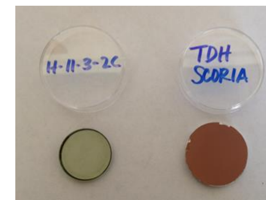
Figure 5. Examples of Glass Fusions and Pressed Pellets used in experimentation.
