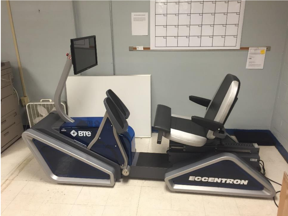
Appendix 2. BTe Eccentron Trainer. Participant sits and has feet strapped to pedals. The computer records average values of resistance and observers record peak values during training.
