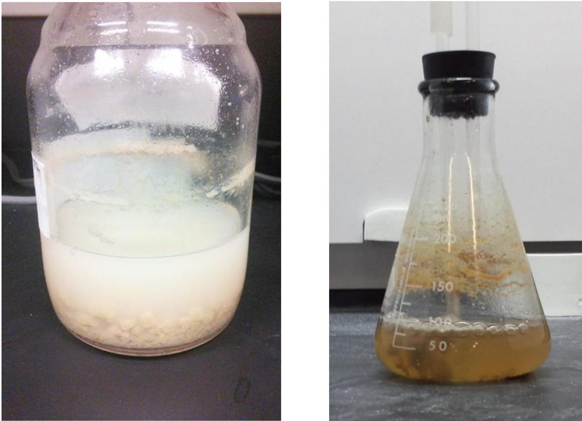
**Figure 11:** Comparison of liquid suspension culture performance between shaker culture (left, shaker not pictured) and experimental bubble bioreactor (right) in terms of media coloration. Picture taken roughly 40 days after inoculation.
