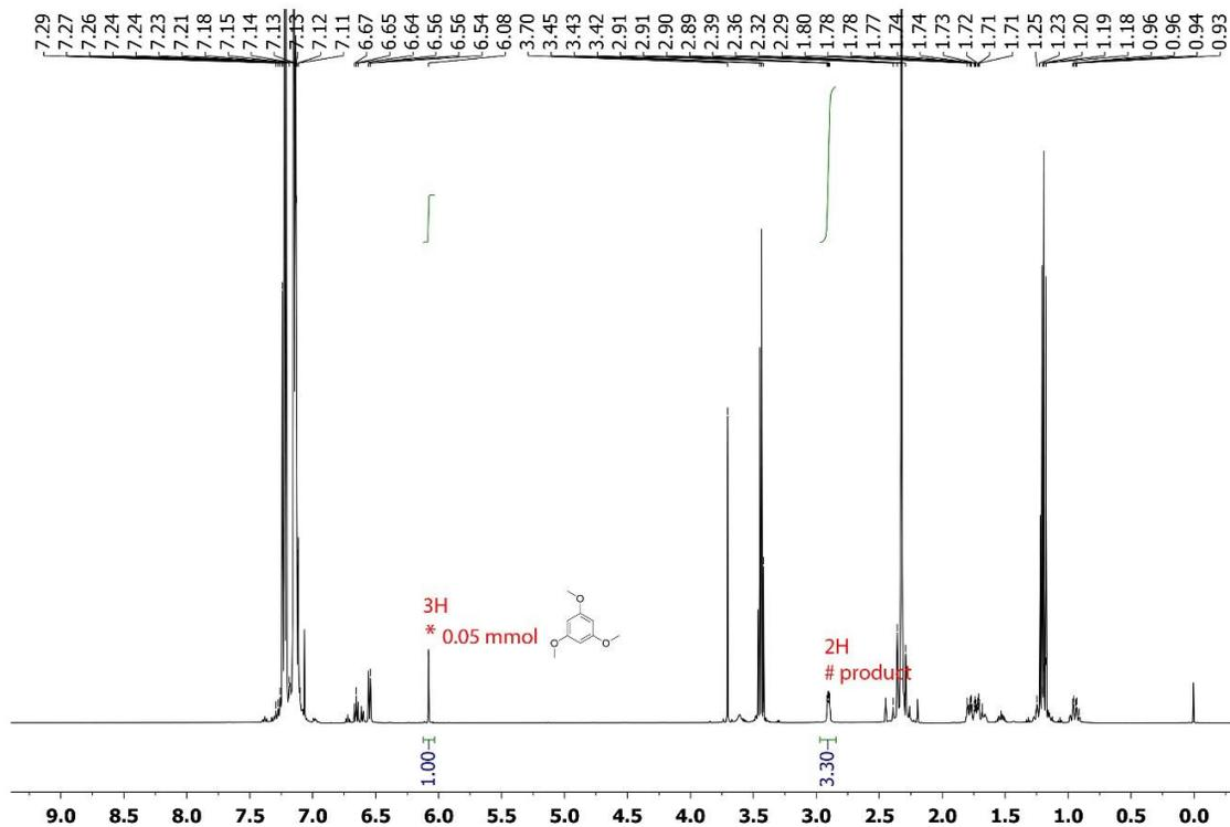
Figure 2.68.  $^1\text{H}$  NMR (500 MHz,  $\text{CDCl}_3$ ) of the reaction mixture of 4ac.
