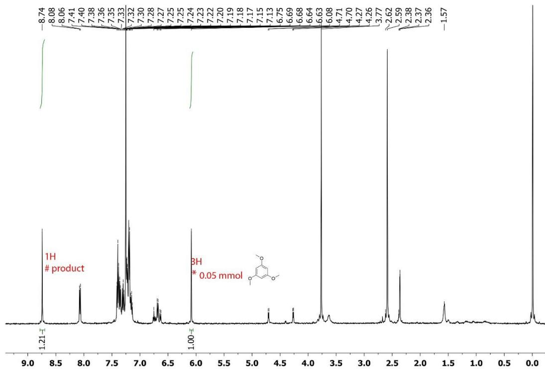
Figure 2.35  $^1\text{H}$  NMR (500 MHz,  $\text{CDCl}_3$ ) of the reaction mixture of 3r.
