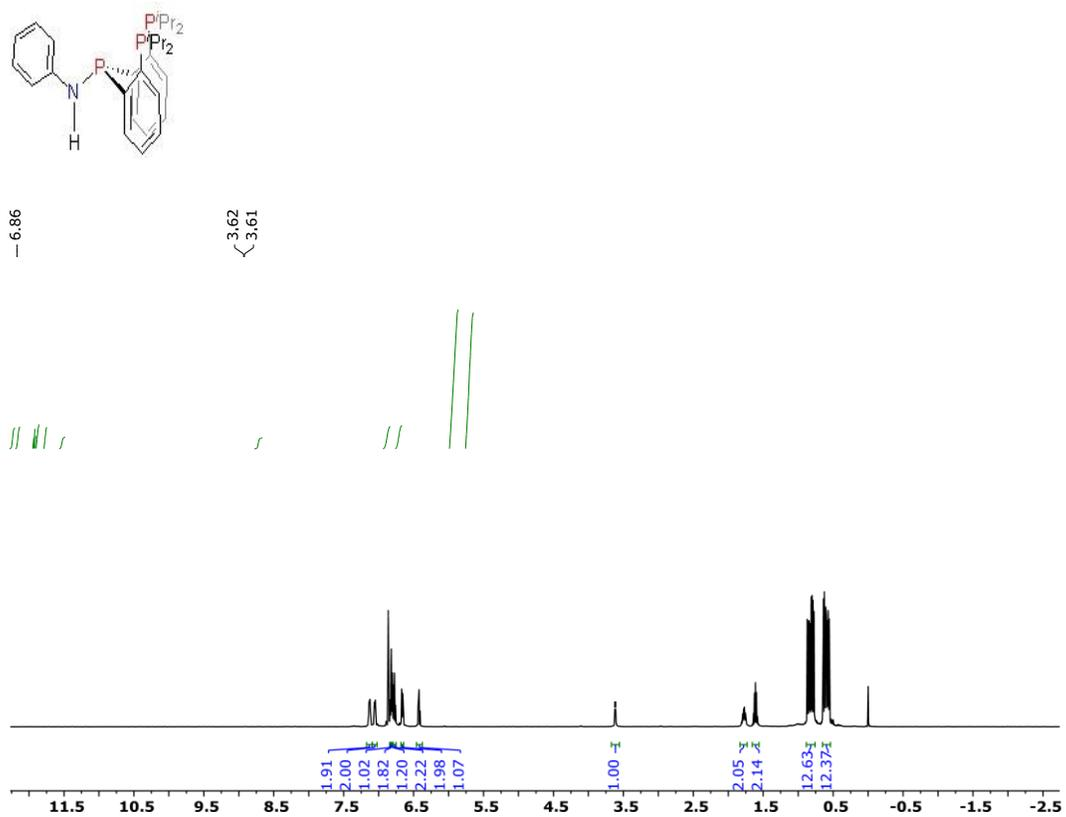
Figure 2.76  $^1\text{H NMR}$  (500 MHz,  $\text{C}_6\text{D}_6$ ) of IV ligand.
