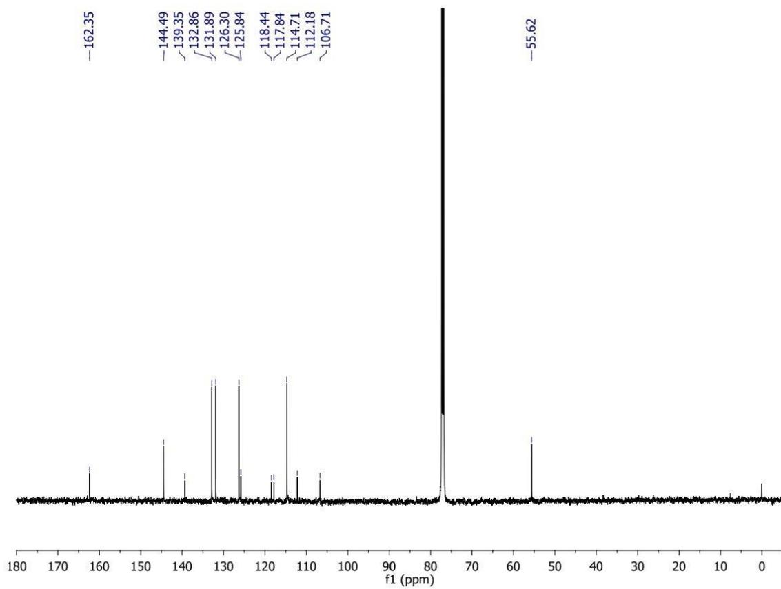
Figure 4.46  $^{13}\text{C}$  NMR ( $\text{CDCl}_3$ , 125 MHz) of 3t
