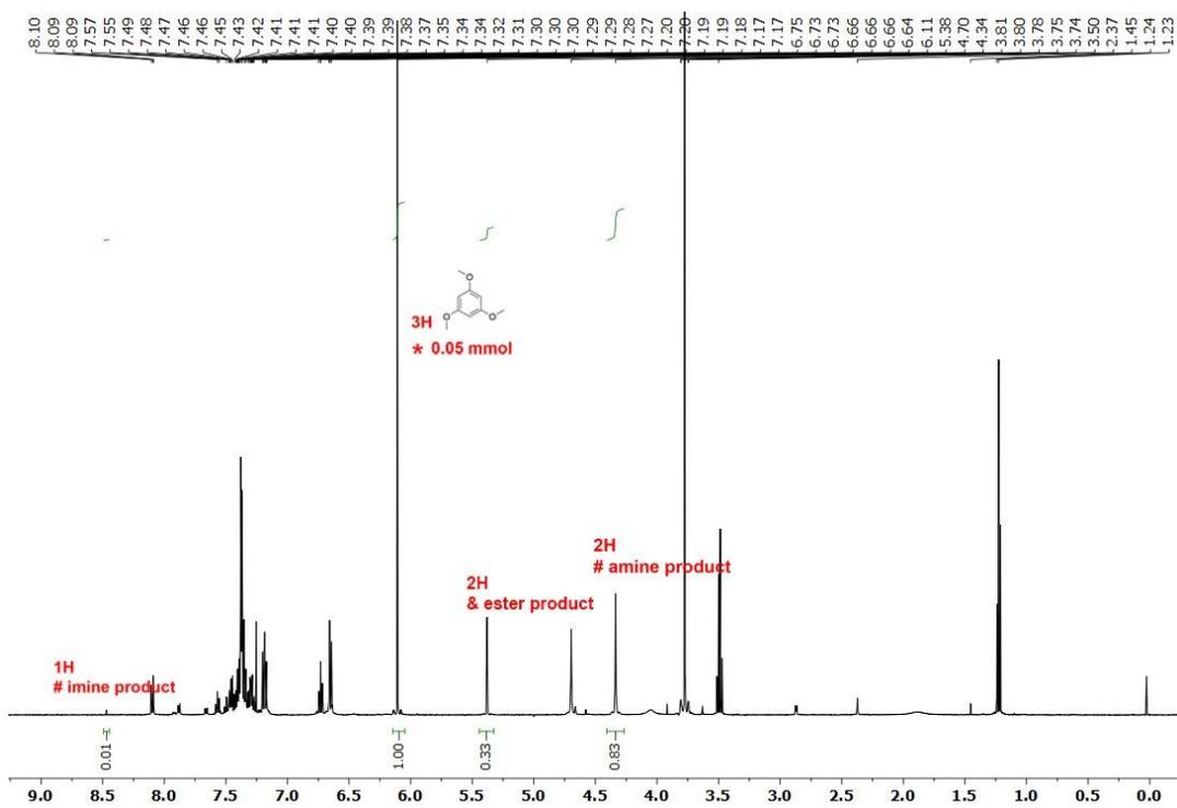
Figure 2.11  $^1\text{H}$  NMR (500 MHz,  $\text{CDCl}_3$ ) of the reaction mixture of imine synthesis by III and  $\text{KO}^t\text{Bu}$ .
