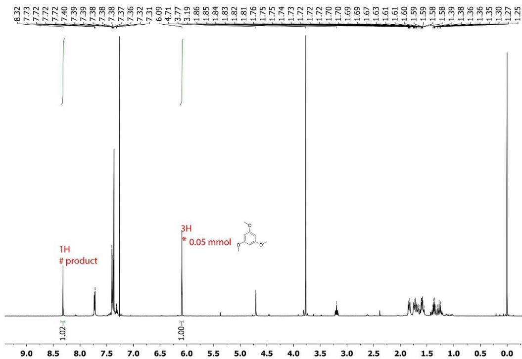
Figure 2.41  $^1\text{H}$  NMR (500 MHz,  $\text{CDCl}_3$ ) of the reaction mixture of 3x.
