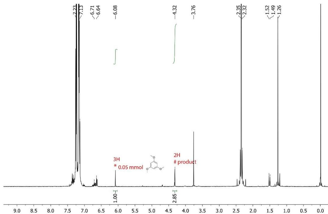
Figure 2.18  $^1\text{H}$  NMR (500 MHz,  $\text{CDCl}_3$ ) of the reaction mixture of amine synthesis by VI and  $\text{KO}^t\text{Bu}$ .
