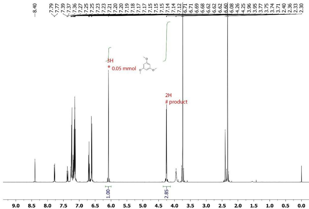
Figure 2.47  $^1\text{H}$  NMR (500 MHz,  $\text{CDCl}_3$ ) of the reaction mixture of 4b.
