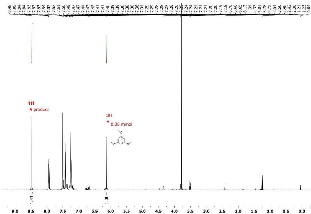
Figure 2.9  $^1\text{H}$  NMR (500 MHz,  $\text{CDCl}_3$ ) of the reaction mixture of imine synthesis by II and  $\text{KO}^t\text{Bu}$ .
