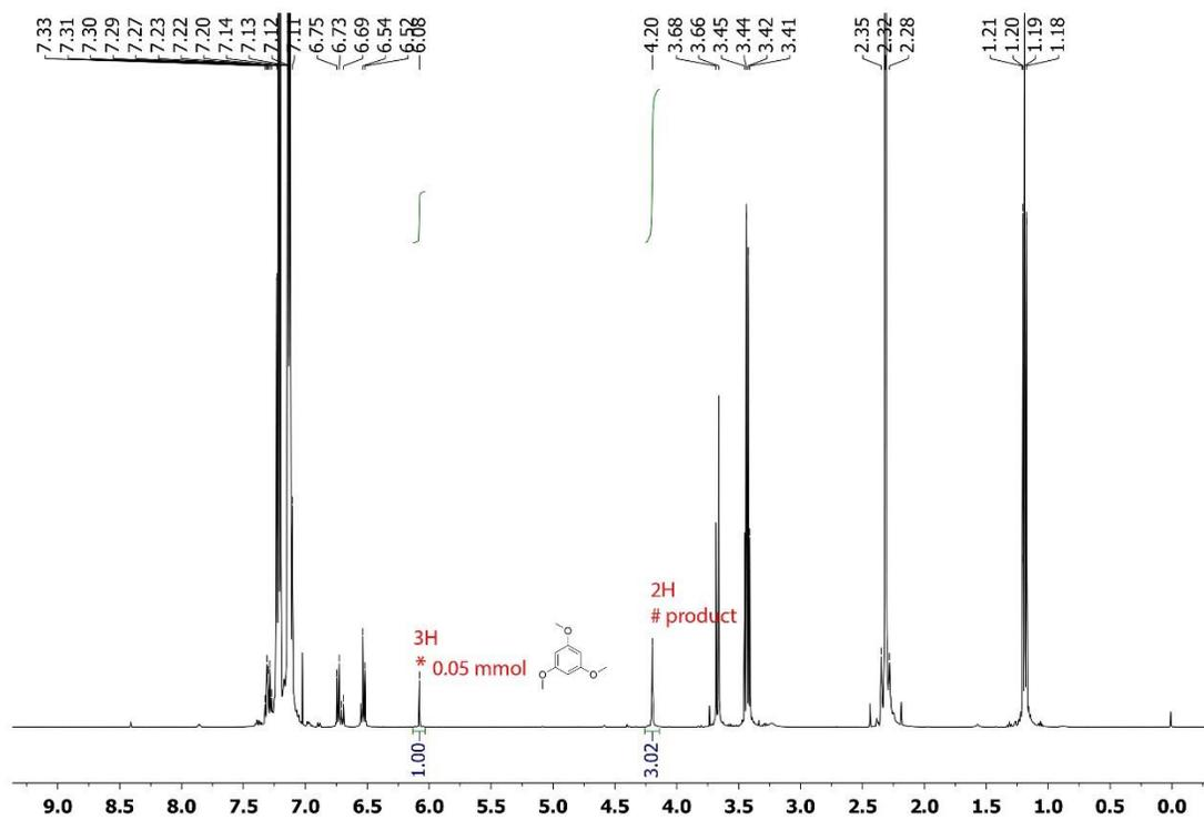
Figure 2.53  $^1\text{H}$  NMR (500 MHz,  $\text{CDCl}_3$ ) of the reaction mixture of 4h.
