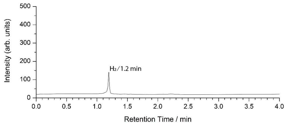
Figure 2.1 H<sub>2</sub> detection by GC chromatography.
