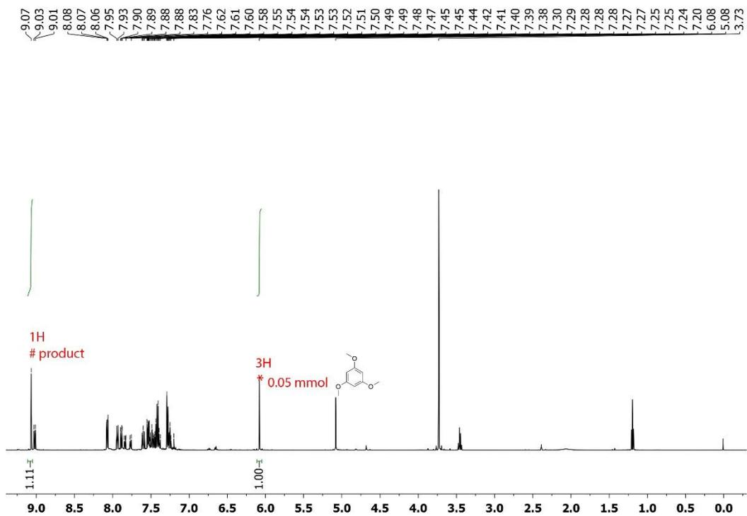
Figure 2.37  $^1\text{H}$  NMR (500 MHz,  $\text{CDCl}_3$ ) of the reaction mixture of 3t.
