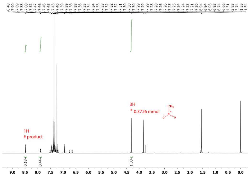
Figure 2.24  $^1\text{H}$  NMR (500 MHz,  $\text{CDCl}_3$ ) of the reaction mixture of 3g.
