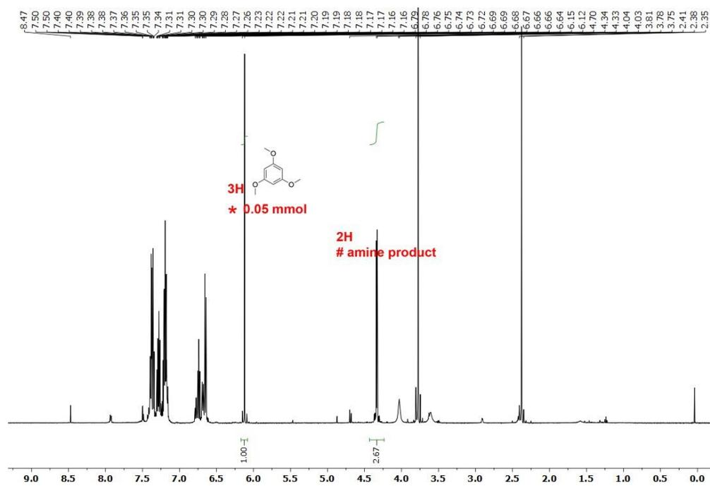
Figure 2.12  $^1\text{H}$  NMR (500 MHz,  $\text{CDCl}_3$ ) of the reaction mixture of amine synthesis by III and  $\text{KO}^t\text{Bu}$ .
