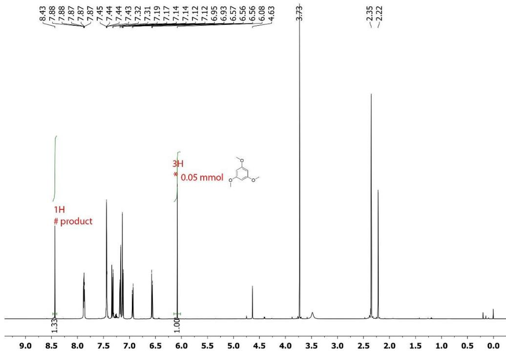
Figure 2.20.  $^1\text{H}$  NMR (500 MHz,  $\text{CDCl}_3$ ) of the reaction mixture of 3c.
