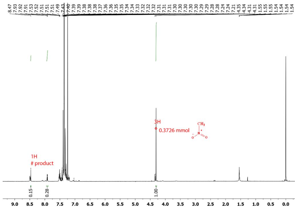
Figure 2.40  $^1\text{H}$  NMR (500 MHz,  $\text{CDCl}_3$ ) of the reaction mixture of 3w.
