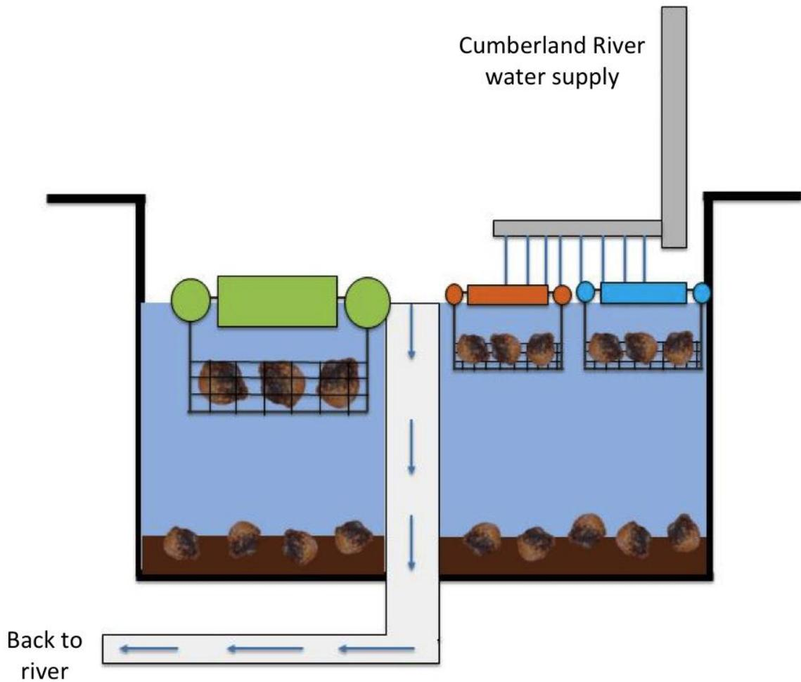
**Figure 1:** Tank set up in the C-RAC. Rectangles and circles represent pool noodles. The black lines underneath them represent PVC floating baskets. Water from the Cumberland River flows from the water supply into the tank from above and through 13 holes and exits through an overflow drainpipe back to the same River.
