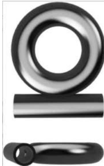
FIGURE 4: Two views of the ring resonator structure. In all rings used in these experiments, the inner opening diameter was 2.0cm. For the single ring results, the ring radius was 9.0 cm to the centerline of the circular waveguide. For the add-drop experiments, the ring diameter was 8.0cm. For the ring array, the diameter is 4.5 cm. The lower figure illustrates the opening that connected the ring and straight waveguides.
