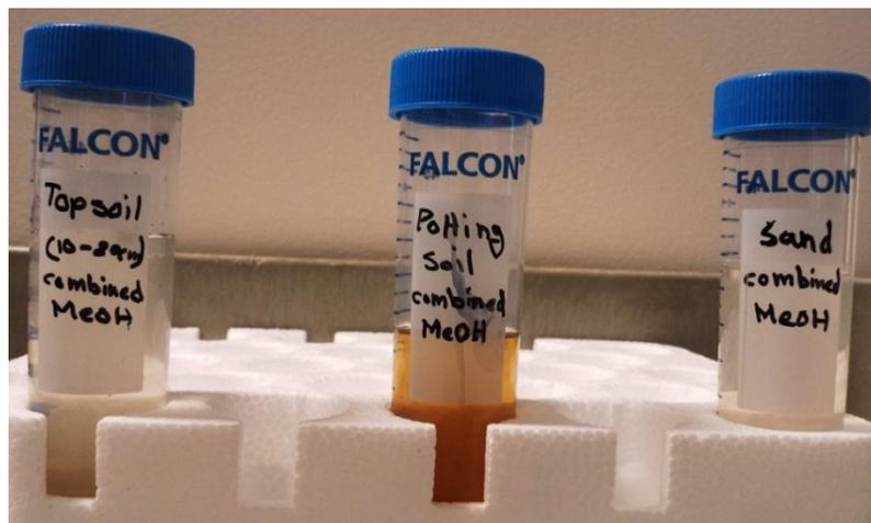
**Figure 7:** Combined 35 mL of methanol solution was centrifuged at 4000 rpm for 30 minutes to remove particulate matter.
