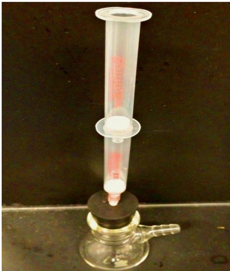
**Figure 10:** A second SPE cartridge was attached to determine if analyte breaks through the first SPE cartridge during the adsorption phase.
