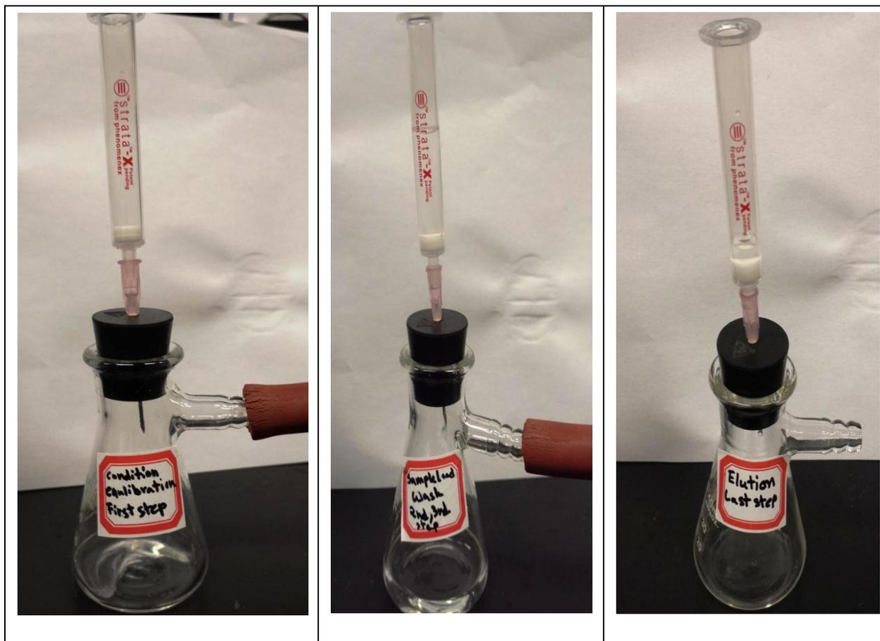
**Figure 9:** Solid phase extraction process in steps utilizing Strata-X 33µm polymeric reverse phase extraction cartridges.
