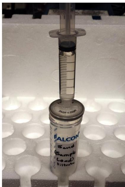
**Figure 8:** Filtration through a Millex – GV PVDF 0.22  $\mu\text{m}$  syringe driven filter to remove any particulate matter.
