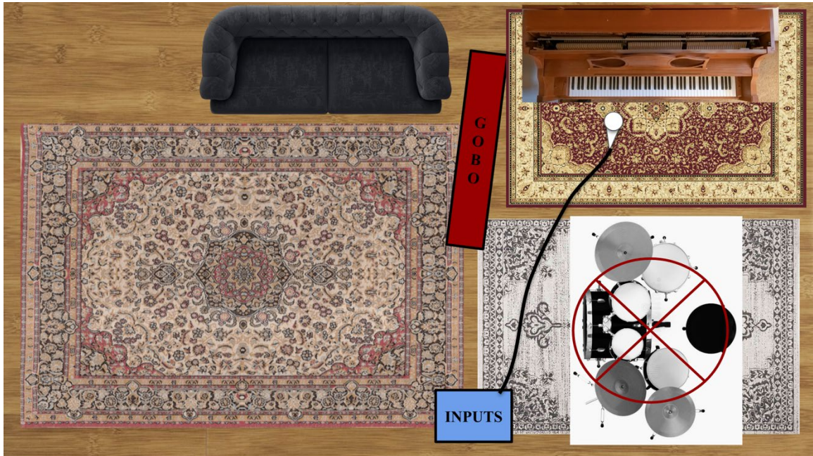
Figure 7. Placement of instruments, microphones, and other equipment used for the sixth and final phase of “modern” recording. Not to scale.
