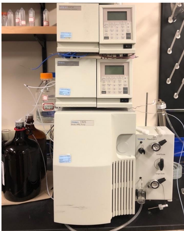
Figure 2.5 Waters 1525 Binary HPLC Pump with Waters 2489 UV/Visible Detector
